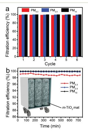
Fig. 6 PM removal efficiencies of the  $Au@m-TiO_2$  mat (a) over six cycles and (b) for the outdoor long-term filtration process. The inset in (b) shows the schematic illustration of a portable, high-temperature resistant, recyclable air-purification device integrated with the  $m-TiO_2$  mat.
