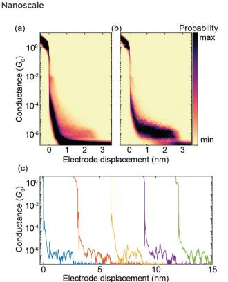
**Fig. 6** Fast-breaking measurement of PC1. (a) 2D conductance-displacement density plot consisting of 10 000 consecutive fast-breaking traces. (b) 2D histogram containing only molecular traces, obtained through a reference-free clustering algorithm.<sup>21</sup> (c) Five examples of individual breaking traces, each displaced by hand by 3 nm to ensure good visibility.
