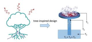
evaporator design for reducing heat loss
