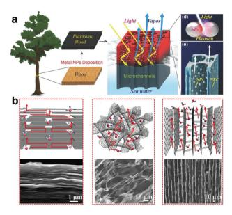
Fig. 4 Water transport. (a) Schematic illustration of a plasmonic-woodbased evaporator. This figure has been reproduced from ref. 56 with permission from WILEY-VCH Verlag GmbH & Co. KGaA, Weinheim, copyright 2017. (b) Mechanism of the water transport channels of VA-GSM (right) and other rGO materials. This figure has been reproduced from ref. 18 with permission from American Chemical Society, copyright 2017.
