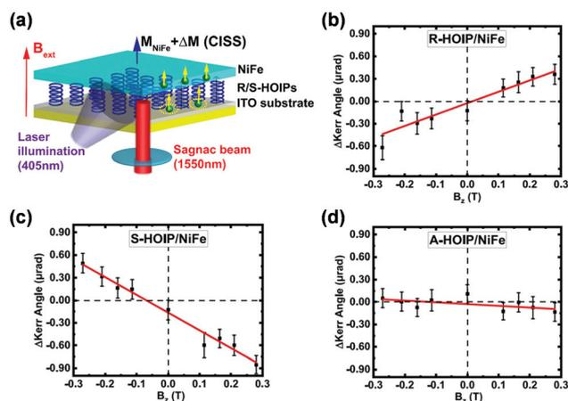
**Fig. 9** (a) Schematic illustration of Sagnac MOKE experiment for the light-driven CISS effects-induced interfacial magnetization. (b–d) The measured Kerr signals upon laser illumination for (b) *R*-MBA<sub>2</sub>PbI<sub>4</sub>/NiFe, (c) *S*-MBA<sub>2</sub>PbI<sub>4</sub>/NiFe and (d) achiral MBA<sub>2</sub>PbI<sub>4</sub>/NiFe under positive/negative external magnetic field. This figure has been adapted/reproduced from ref. 109 with permission from American Chemical Society, Copyright 2020.
