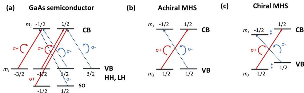
**Fig. 4** Spin-dependent optical transitions in GaAs, achiral MHS and chiral MHS.
