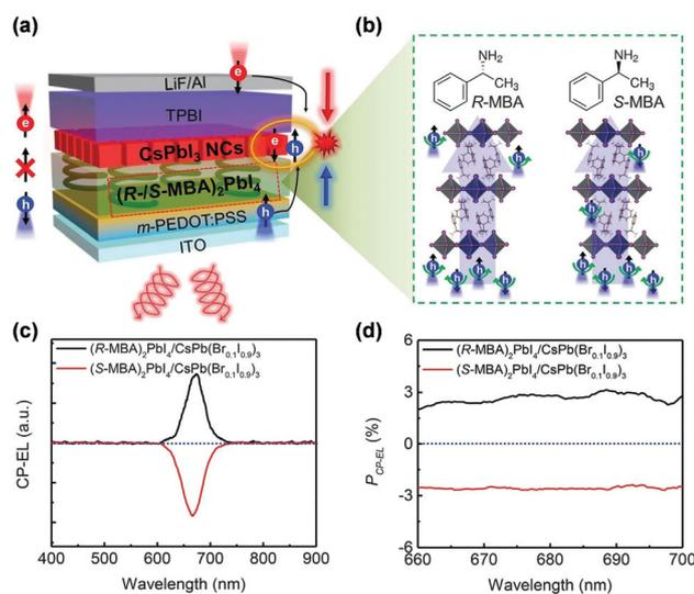
Fig. 13 (a) Schematic illustration of spin-polarized charge injection and CP-EL emission in spin-LED. (b) The structures of chiral  $R\text{-}/S\text{-MBA}$  molecules and 2D  $(R\text{-}/S\text{-MBA})_2\text{PbI}_4$  perovskites. (c) The CP-EL spectra and (d) EL polarization degree ( $P_{\text{CP-EL}}$ ) of spin-LED based on CISS layer/ $\text{CsPbI}_3$  NCs heterostructures. This figure has been adapted/reproduced from ref. 113 with permission from Science, Copyright 2021.
