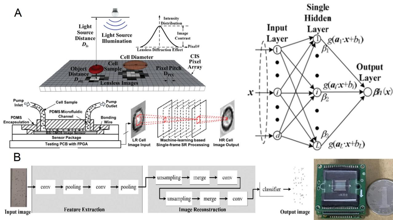
**Fig. 1** (A) Schematic diagram of the lens-free cell counting system and model structure of the extreme learning machine. Reproduced from ref. 68 with permission from Molecular Diversity Preservation International, 2016. (B) Cell division network structure in lensless imaging systems and comparison between the microfluidic chip and a coin. Reproduced from ref. 69 with permission from Molecular Diversity Preservation International, 2019.
