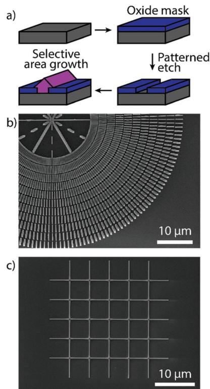
**Fig. 1** (a) Schematic of the SAE growth process for  $\text{Zn}_3\text{P}_2$ . (b) Overview SEM image of  $\text{Zn}_3\text{P}_2$  nanowires grown at different angles by SAE. (c) SEM image of a  $\text{Zn}_3\text{P}_2$  nanowire network grown by SAE.
