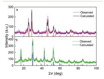
Fig. 1 XRD diffractograms of (a)  $GdF_3@EG$  and (b)  $GdF_3@PSSMA$  nanoparticles and comparison with calculated patterns. The vertical lines indicate diffractions of the hexagonal (red) and orthorhombic  $LnF_3$  phases (blue). The original data retrieved from Inorganic Crystal Structure Database were based on the  $P6_3/mcm$  of  $CeF_3$  no. 42470 and Pnma of  $EuF_3$  no. 95244 reflected by calculated patterns no. 01-074-3116 and 01-089-1933 in PDF, respectively.
