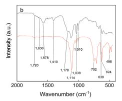
Fig. 3 FTIR spectra of PSSMA (black), GdF<sub>3</sub>@EG (blue), GdF<sub>3</sub>@PSSMA (red), and GdF<sub>3</sub>@PSSMA-PSDA-A488 nanoparticles (green).
