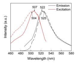
**Fig. 4** Photoluminescence spectra of PSDA-A488 (dotted line) and GdF<sub>3</sub>@PSSMA-PSDA-A488 nanoparticles (solid line).
