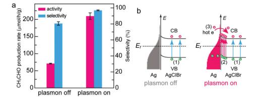
Fig. 4 Plasmonic effect on the photocatalytic performance. (a) Comparison of the photocatalytic  $CH_3CHO$  production activity and selectivity of the Janus  $Ag/AgCl_{0.79}Br_{0.21}$  nanostructures under different light irradiation. (b) Plasmonic effect on the hot carrier generation.  $E_f$ , Fermi level; CB, conduction band; VB, valence band.
