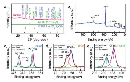
Fig. 2 Structure and composition of the Janus Ag/AgClBr nanostructures. (a) XRD patterns of the Janus Ag/AgCl<sub>0.79</sub>Br<sub>0.21</sub> nanostructures. XPS survey spectrum (b) and high-resolution Ag 3d (c), Br 3d (d), and Cl 2p (e) XPS spectra of the Janus Ag/AgCl<sub>0.79</sub>Br<sub>0.21</sub> nanostructures.
