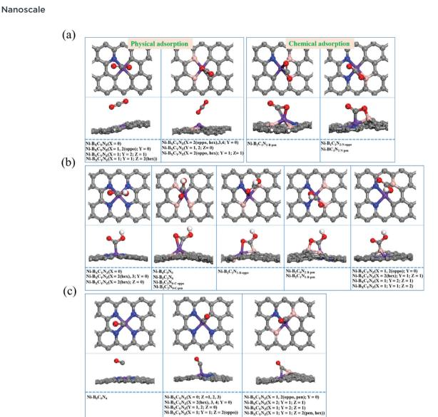
Fig. 3 The different adsorption modes of \*CO $_2$  (a), \*COOH (b), and \*CO (c) intermediates on Ni-B $_X$ C $_Y$ N $_Z$ .
