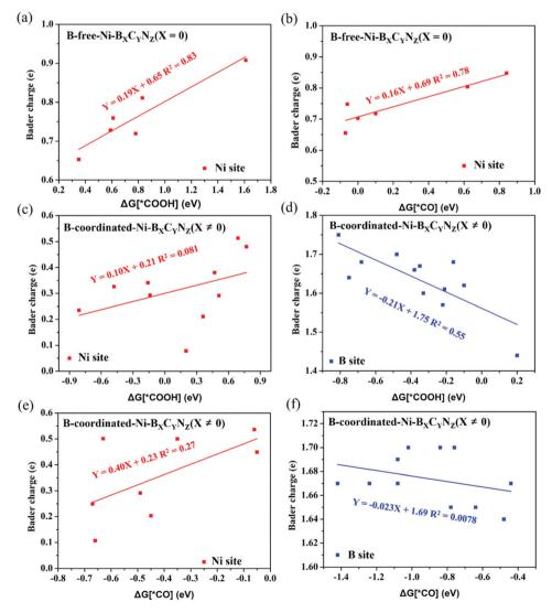
Fig. 6 Bader charge analysis of active sites (Ni or B atom) on \*COOH and \*CO adsorbed Ni $-B_XC_YN_Z$ . Correlations of the adsorption free energy of \*COOH (a) and \*CO (b) intermediates with Ni Bader charge on B-free Ni $-B_XC_YN_Z$  (X=0). Correlations of the adsorption free energy of \*COOH and \*CO intermediates with Ni (c, e) and B Bader charge (d, f) on B-coordinated Ni $-B_XC_YN_Z$  ( $X\neq0$ ).
