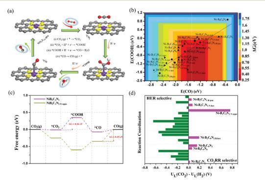
Fig. 5 Schematic of the four-step reaction processes of CO<sub>2</sub> reduction to CO on Ni-B<sub>X</sub>C<sub>Y</sub>N<sub>Z</sub> (a). 2D volcano plot for CO evolution on Ni-B<sub>X</sub>C<sub>Y</sub>N<sub>Z</sub> catalysts (b). Free energy diagrams for the  $CO_2RR$  on  $Ni-B_0C_3N_1$  and  $Ni-B_1C_1N_{2-N-oppo}$  (c). The limiting potential difference between  $CO_2$  reduction  $(U_L(CO_2))$  and HER  $(U_L(H_2))$  on various Ni-B<sub>X</sub>C<sub>Y</sub>N<sub>Z</sub> catalysts (d).
