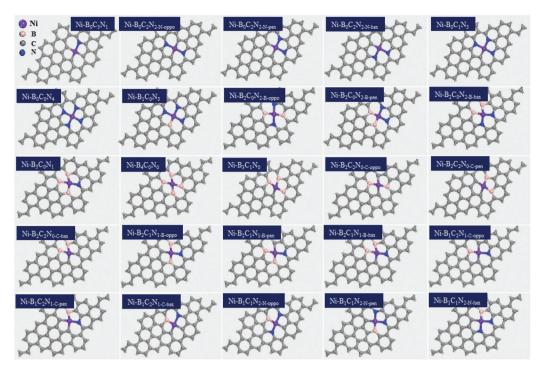
Fig. 2 The optimized structures (top view) of the screened 25 Ni-B<sub>X</sub>C<sub>y</sub>N<sub>z</sub> (X + Y + Z = 4), the color modes: purple for Ni, pink for B, blue for N, and grey for C.
