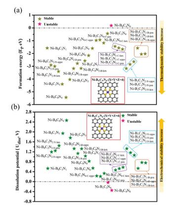
Fig. 1 The DFT-computed formation energy (a) and dissolution potential (b) of  $Ni-B_xC_yN_z$  (X+Y+Z=4). The inset shows the top view of the catalyst model, where the highlighted yellow atoms represent the coordination atoms of the Ni center (purple atom).
