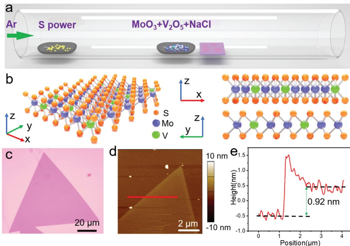
**Fig. 1** (a) Schematic of synthesis of V-doped MoS<sub>2</sub> by CVD. (b) Atom structure and side view of V-doped MoS<sub>2</sub>. (c) Optical image of a V-doped MoS<sub>2</sub> single crystal. (d and e) AFM topography and thickness measurement of V-doped MoS<sub>2</sub>.
