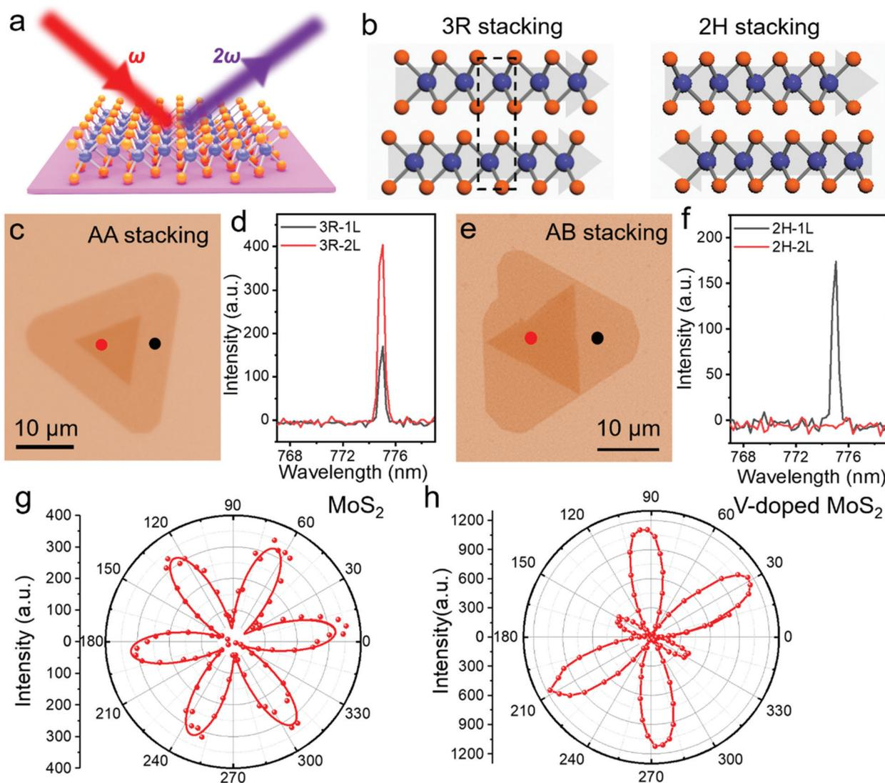
Fig. 4 (a) Schematic diagram of SHG process. (b) Side view of bilayer 3R and 2H phase MoS<sub>2</sub> with different stacking order. (c and e) Optical images of MoS<sub>2</sub> with 3R and 2H stacking. (d and f) Layer number-dependent SHG response 3R and 2H phase V-doped MoS<sub>2</sub>. (g and h) Angular-dependent SHG intensity of monolayer MoS<sub>2</sub> and V-doped MoS<sub>2</sub>.
