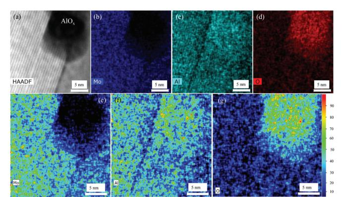
Fig. 1 (a) HAADF STEM image of MoAlB-MoB-AlO<sub>x</sub> heterostructures near an AlO<sub>x</sub> oxide feature and (b-d) Mo (blue), Al (cyan) and O (red) elemental distribution maps from EDX of the same region. (e)–(g) Relative elemental intensity distributions of Mo, Al and O within the area; red signifies highest, blue lowest intensity.
