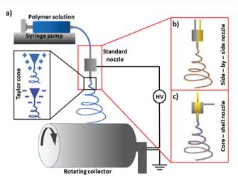
Fig. 3 Scheme of electrospinning with (a) a standard nozzle; (b) a sideby-side nozzle; (c) a co-axial nozzle, showing the principle of the electrospinning process: high voltage is applied to the nozzle and deposition takes place on the collector, which is presented here as a rotating drum.
