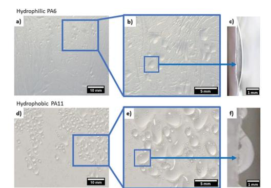
Fig. 7 Comparing the shape of droplets collected on the electrospun (a–c) hydrophilic PA6 and (d–f) hydrophobic PA11 meshes. Adapted and reproduced with permission. 161
