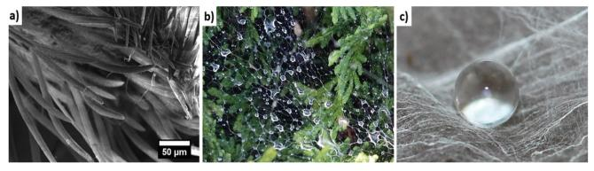
Fig. 2 (a) Scanning electron microscopy (SEM) micrograph of spider spinnerets of *Grammostola pulchra*; (b) photograph of water droplets captured on a spider web in nature; (c) the water droplet deposited on a *Linothele Megatheloides* web that was wrapped around a piece of wood, evidencing the superhydrophobic property of this web.
