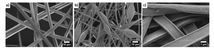
Fig. 4 SEM micrographs showing electrospun PS fibers: (a) smooth and uniform; (b) with beads; (c) gutter shape PS-CA fibers produced with a side-by-side nozzle.
