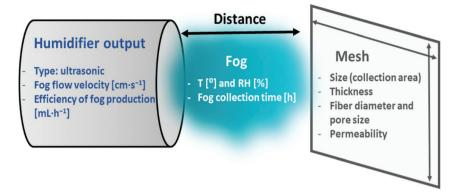
Fig. 11 The graphic illustration of the most important fog collection parameters in laboratory-scale experiments.
