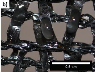
Fig. 1 Images of (a) a typical double layer of a Raschel mesh and (b) water droplets collected on a Raschel mesh
