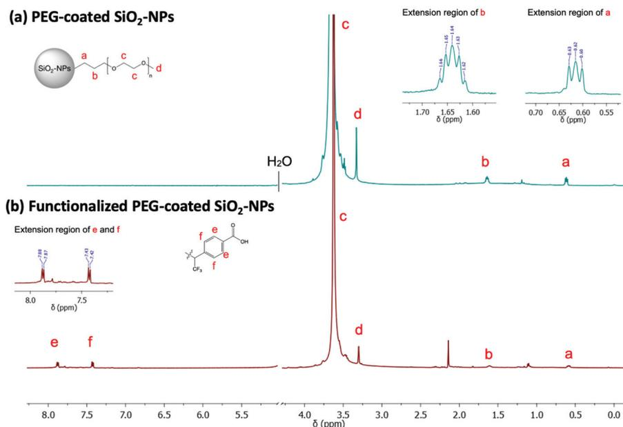
Fig. 3 Stacked  $^1\text{H}$  spectra of empty PEG-coated silica nanoparticles ( $\text{D}_2\text{O}$ , 500 MHz).  $^1\text{H}$  NMR spectrum (a) before and (b) after photografting (365 nm, 45 min) and purification step. NMR peak at 2.2 ppm (bottom spectrum) arises from acetone.
