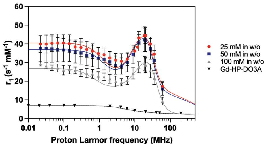
Fig. 5 NMRD profiles ( $T = 37\text{ }^{\circ}\text{C}$ ) obtained for the paramagnetic complexes entrapped on PEG-coated  $\text{SiO}_2$ -Gd-NPs (16, 18 and 25 nm) as a result of [Gd-HP-DO3A] in w/o procedure (triangles, squares and squares on edge, respectively) and free Gd-HP-DO3A complex (circles) in aqueous solution. Longitudinal ( $r_1$ ) relaxometric measurements plots are normalized per paramagnetic gadolinium ion concentration ( $\text{s}^{-1}\text{ mM}^{-1}$ ).
