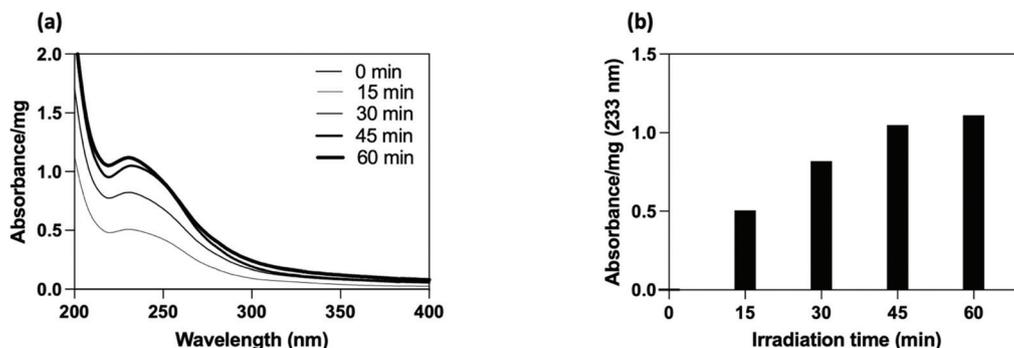
Fig. 2 UV irradiation time study. (a) UV spectra after purification and (b) plot result of the linker absorbance (233 nm) on PEG-coated  $\text{SiO}_2$ -NPs normalized per mg of particles for different time of exposure.
