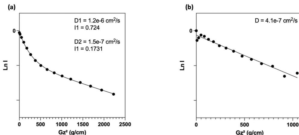
Fig. 1 DOSY-NMR experiments. Semilogarithmic plot of echo intensity vs. the square of the gradient strength recorded on PEGylated  $\text{SiO}_2$ -NP systems after dialyzing the samples (a) at room temperature; (b) at 35 °C.
