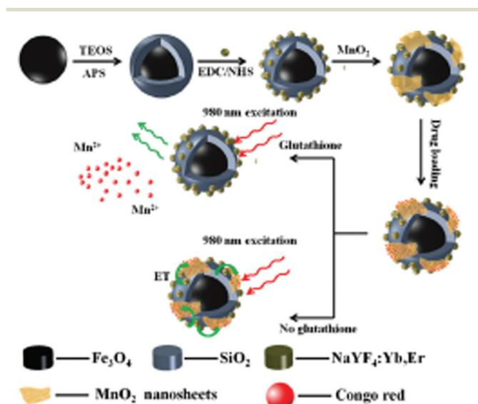
Fig. 1 Schematic illustration of the synthetic procedure for the preparation of the MSU/MnO<sub>2</sub>-CR drug delivery system. Reprinted with permission from ref. 122 Zhao *et al.*, *Dalton Trans.*, 2014, 43, 451–457. Copyright©2014, The Royal Society of Chemistry.
