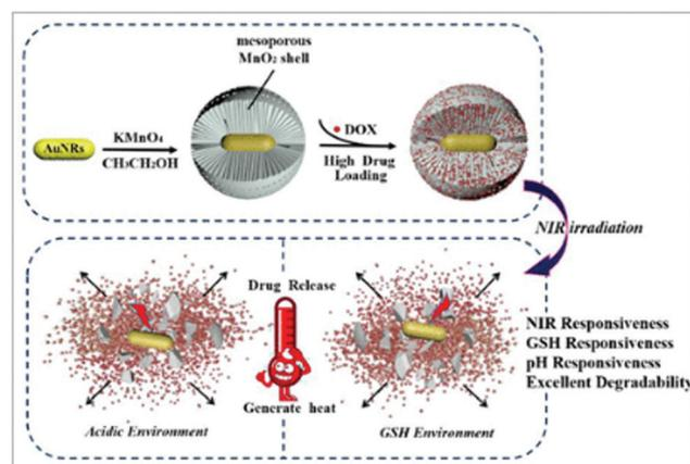
**Fig. 3** Scheme of the preparation of Au/ $MnO_2$  nanoparticles and drug release of Au/ $MnO_2$  nanoparticles. Reprinted with permission from ref. 135 Zhang *et al.*, *Eng. Chem. Res.*, 2019, **58**, 2991–2999. Copyright©2019, the American Chemical Society.
