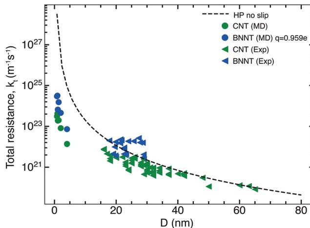
**Fig. 3** Variation of total resistance  $k_t$  for one nanotube with diameter compared between our MD and experiments. Data from the experimental membranes have been scaled to reflect the resistance of a single nanotube.<sup>13,36</sup> Comparisons are made with MD simulations of the smallest diameters and the no slip HP equation. All membranes considered have been scaled to 50  $\mu\text{m}$ . Entrance/exit resistances  $k_1$  are negligible.
