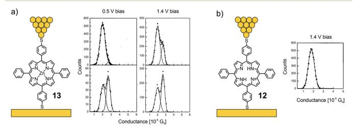
Fig. 6 Left: Chemical structures of 13 (a) and 12 (b) depicted in an STM-BJ. Right: 1D-histograms of bistable 13 at 500 and 1400 mV bias (a) and 1D-histogram of 12 at 1400 mV bias (b), adapted from ref. 53 with permission from the American Institute of Physics.
