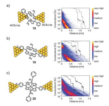
Fig. 8 Left: Chemical structures of 18 (a), 19 (b), and 20 (c) depicted in an MCBJ. Right: Corresponding 2D-conductance vs. displacement histograms with off-set exemplary single-traces showing the high-conductance (HC) medium conductance (MC) and low conductance (LC) molecular features, adapted from ref. 55 with permission from John Wiley and Sons.
