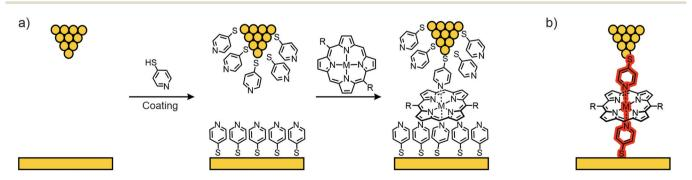
Fig. 13 (a) Electrode coating demonstrated using 4-thiopyridine followed by deposition of a metal porphyrin. (b) Envisioned CPP transport pathway through the electrode-coordinated porphyrin plane, highlighted in red.
