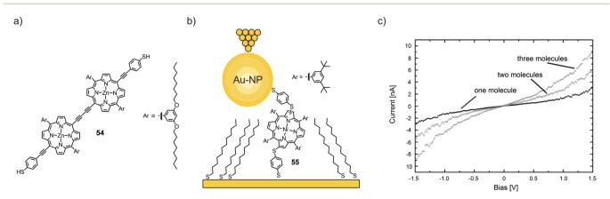
Fig. 20 (a) Chemical structure of 54. (b) Chemical structure of 55 depicted in a thioalkane self-assembled monolayer (SAM) with opposite tipcontact via a chemisorbed gold nanoparticle (Au-NP) in an STM-BJ. (c) Three distinct I(V) characteristics observed for the junctions depicted in (a) corresponding to one, two, or three molecules bridging the circuit in parallel, adapted from ref. 75 with permission from The Royal Society of
