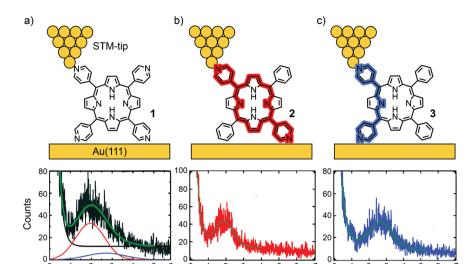
Fig. 3 Upper: Chemical structures of 1 (a), 2 (b), and 3 (c) depicted in an STM-BJ. Lower: 1D-histograms of molecular junctions formed by 1 (a), 2 (b), and 3 (c), adapted with permission from ref. 48. Copyright 2012 American Chemical Society. The "para-pathway" is highlighted in red and the "ortho-pathway" in blue.
