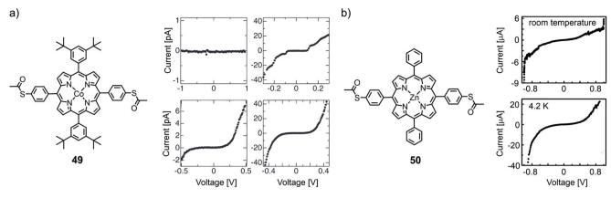
Fig. 17 (a) Chemical structure of 49 (left) and four different observed I(V) curves at 11 K (right), as adapted from ref. 68 (permission from the Japanese Society of Applied Physics is currently under request). (b) Chemical structure of 50 (left) and molecular I(V) curves at room temperature and 4.2 K (right), adapted from ref. 69 with permission from the American Institute of Physics.
