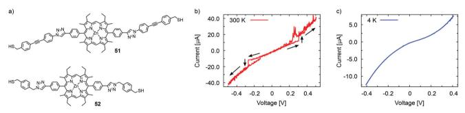
Fig. 18 (a) Chemical structures of 51 and 52. /(V) traces recorded with an electromigrated molecular junction with immobilized 51 at (b) 300 K and at (c) 4 K. The bistability in (b) at  $\pm 0.3$  V was observed with a voltage sweep of  $0 \rightarrow -0.5 \rightarrow 0.5 \rightarrow 0$  (V). The I(V) curves of (b) and (c) are adapted with permission from ref. 70. Copyright 2015 American Chemical Society.
