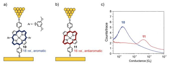
Fig. 5 Chemical structures of porphyrin 10 (a) and norcorrole 11 (b) depicted in an STM-BJ. The 18 π-electron aromatic macrocycle in 10 is highlighted in blue and the 16  $\pi$ -electron antiaromatic macrocycle in 11 is highlighted in red. (c) 1D-histogram of molecular junctions of 10 and 11, adapted form ref. 50 with permission from Springer Nature.
