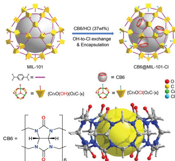
**Scheme 1** Top: Schematic representation of the encapsulation of CB6 molecules in MIL-101 with the formation of the CB6@MIL-101-Cl composite. The two coordinated aqua ligands on the trinuclear chromium SBU are not indicated for clarity. Bottom: Formula and structure of CB6 = cucurbit[6]uril. The yellow sphere represents the intrinsic pore.
