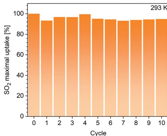
Fig. 5 SO<sub>2</sub> adsorption capacity of CB6@MIL-101-Cl at 293 K and 0.96 bar, measured over 10 repetitive adsorption–desorption cycles.
