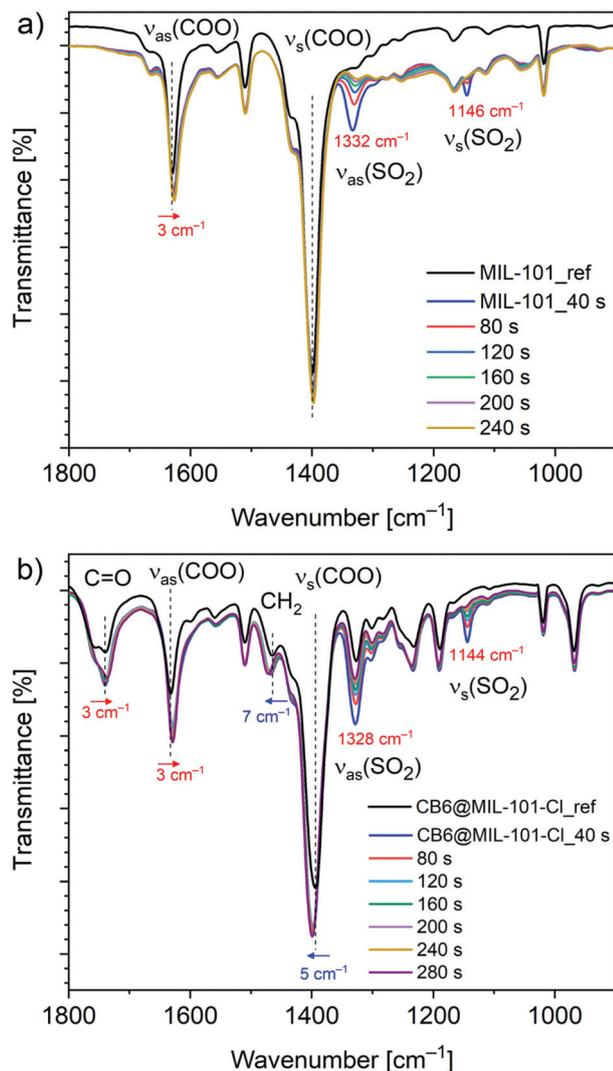
Fig. 4 FT-IR spectra of (a) MIL-101 and (b) CB6@MIL-101-Cl before and after single exposure and loading with SO<sub>2</sub> (see Exp. section for details).
