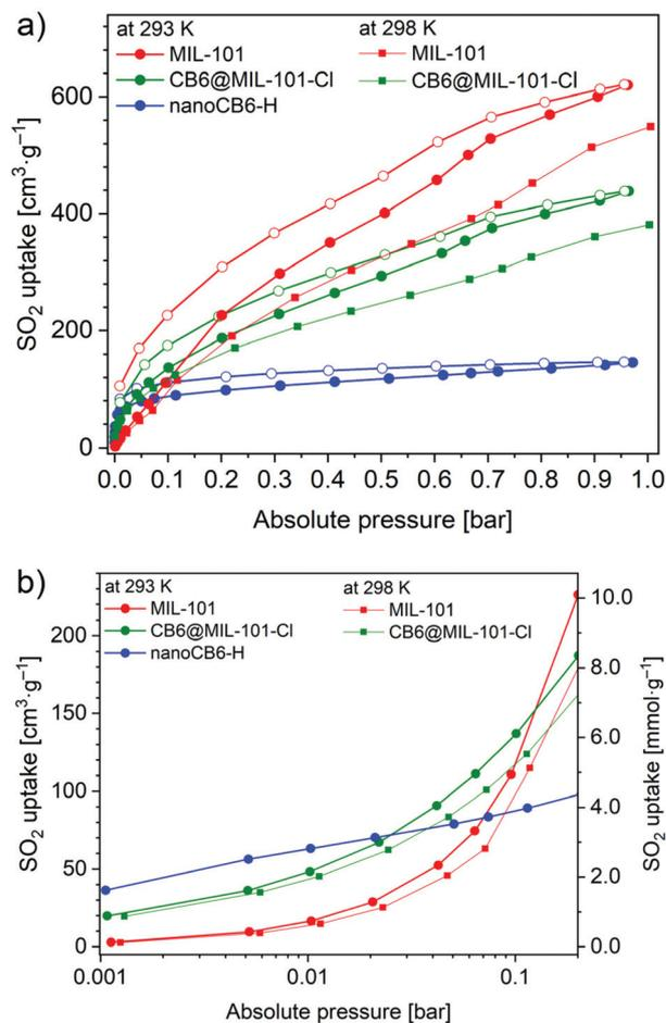
Fig. 2 SO<sub>2</sub> sorption isotherms for MIL-101 and CB6@MIL-101-Cl at 293 K (normal lines) and 298 K (thin lines, adsorption branch only), and for nanoCB6-H at 293 K: (a) 0–1 bar range. (b) 0.001–0.2 range, logarithmic scale (in b the desorption isotherms are omitted for clarity).
