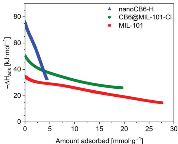
Fig. 3 Isosteric enthalpy of adsorption dependence on the amount of SO<sub>2</sub> adsorbed for MIL-101, CB6@MIL-101-Cl and nanoCB6-H.
