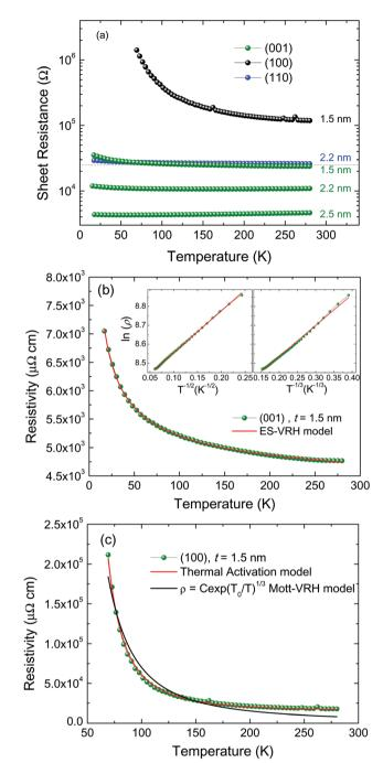
Fig. 5 (a) Sheet resistance calculated for the thinnest (001)- and (100)epitaxial films. (b)  $\rho(T)$  curve for the t = 1.5 nm (001)-epitaxial sample fitted to a ES-VRH model. Inset on the left (right) shows the fit to the ES-VRH model with n = 1/2 (disorder-driven localization 2D Mott-VRH model, n = 1/2) 1/3). (c)  $\rho$ (T) curve for the t=1.5 nm (100)-epitaxial sample fitted to a thermal activation model (red) and a 2D Mott-VRH model (black).
