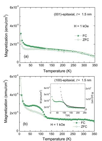
Fig. 7 (a) FC/ZFC M(T) curves measured on the t = 1.5 nm (001)-epitaxial IrO2 film. These curves correspond to H in-plane, but no hint of magnetic order is observed with H out-of-plane. (b) FC/ZFC M(T) curves measured with H applied in-plane on the t = 1.5 nm (100)-epitaxial IrO<sub>2</sub> film. The inset of panel (b) shows a direct comparison to the thermal dependence of the resistivity.
