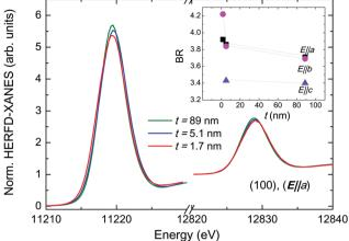
Fig. 3 Comparison of the normalized Ir  $L_{2,3}$ -edges HERFD-XANES spectra recorded on samples with different thicknesses in (100)-epitaxial samples. The inset plots the evolution of the branching ratio with thickness
