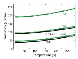
**Fig. 6** Comparison of the representative  $\rho(T)$  curves measured in samples with different substrate-driven strains,  $t \approx 5$  nm (green circles) and  $t \approx 100$  nm (black triangles).
