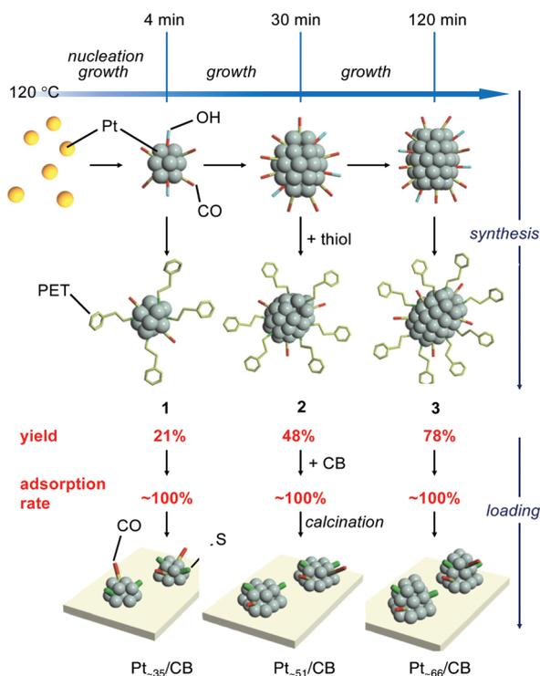
Fig. 4 Proposed mechanism for the synthesis of 1–3 and the preparation of  $Pt_{\sim 35}/CB$ ,  $Pt_{\sim 51}/CB$ , and  $Pt_{\sim 66}/CB$  in the case of loading with 1.0 wt% Pt.
