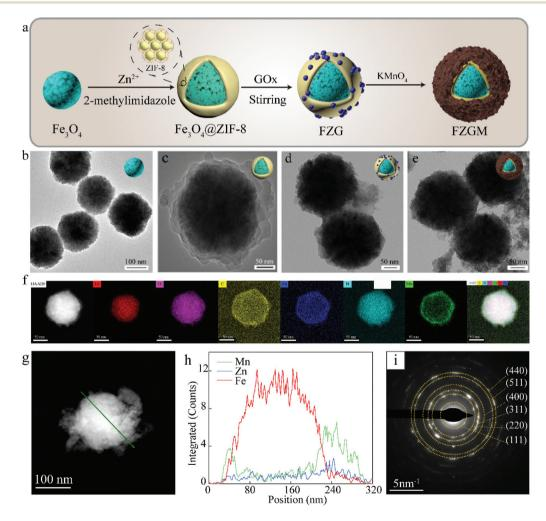
Fig. 1 (a) Schematic diagram of the fabrication process of the FZGM nanozyme. TEM images of (b) Fe<sub>3</sub>O<sub>4</sub>, (c) Fe<sub>3</sub>O<sub>4</sub>@ZIF-8, (d) FZG, and (e) FZGM. (f) HAADF-STEM and elemental mapping images of FZGM. (g and h) Line scan curves of FZGM. (j) SAED diffraction pattern of Fe<sub>3</sub>O<sub>4</sub>.
