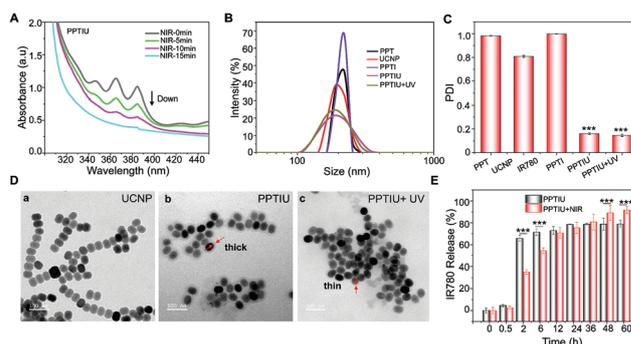
**Fig. 2** (A) The absorbance value of polymeric nanocomposites PPTIU with different times of NIR cross-linking. (B) The particle size and (C) polydispersity index (PDI) of the indicated materials by dynamic light scattering (DLS). (D) The transmission electron microscopy (TEM) analysis in UCNP alone, polymeric nanocomposites with UV irradiation or not. (E) The cumulative IR780 release rate of nanocomposites was determined by HPLC. \*\*\**P* < 0.001 was considered as the significant difference.
