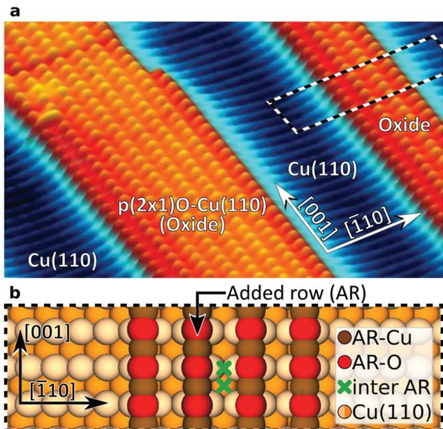
**Fig. 1** Atomic structure of a partially oxidized Cu(110) surface. (a) Constant frequency-shift AFM image of two protruding  $p(2 \times 1)\text{O-Cu}(110)$ -reconstructed oxide stripes (orange) separated by bare Cu(110) areas (blue). (b) Atomistic model of an oxide stripe with four added rows corresponding to the area marked by the dashed box in (a). The green crosses mark distinct atomic sites between the ARs.
