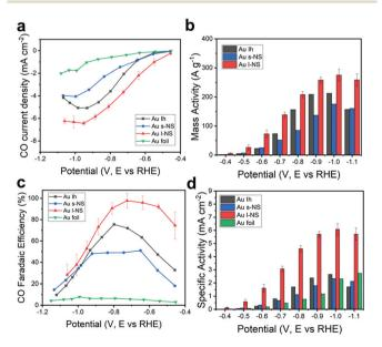
Fig. 2 (a) Partial current densities, (b) mass activities, (c) FEs, and (d) specific activities of Ih (black), s-NS (blue), l-NS (red), and Au foil (green) for CO production versus applied potential.
