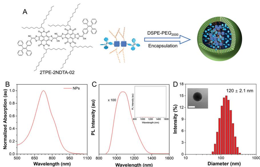
**Fig. 1** (A) Schematic illustrations of fabrication of TN NPs by encapsulating DSPE-PEG<sub>2000</sub> with 2TPE-2NDDTA-02. (B) Normalized absorption spectrum of TN NPs. (C) PL spectra of TN NPs. Concentration: 100  $\mu\text{M}$  (based on TN);  $\lambda_{\text{ex}} = 820 \text{ nm}$ . (D) DLS histogram and TEM image of TN NPs. Scale bar: 100 nm.
