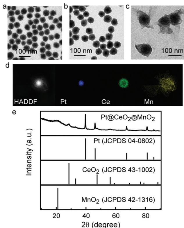
**Fig. 1** TEM images of (a) porous Pt NPs, (b) Pt@CeO<sub>2</sub> and (c) Pt@CeO<sub>2</sub>@MnO<sub>2</sub> nanostructures. (d) STEM images of a single Pt@CeO<sub>2</sub>@MnO<sub>2</sub> nanostructure and elemental mapping images of Pt, Ce and Mn. (e) XRD pattern of the Pt@CeO<sub>2</sub>@MnO<sub>2</sub> nanostructures.
