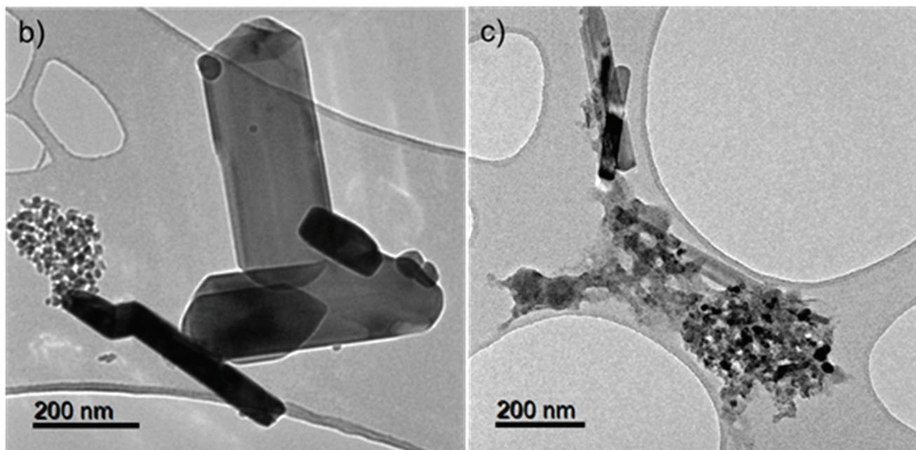
Fig. 1 (a) XRD patterns (Mo-K $\alpha$  radiation) of the  $\text{V}_2\text{O}_5$  and  $\text{V}_2\text{O}_5$ - $\text{TiO}_2$  materials, with an  $\alpha$ - $\text{V}_2\text{O}_5$  reference pattern (PDF 01-072-0433).  $\text{TiO}_2$  diffraction peaks are indicated with asterisks (\*), and the minor impurity peaks assigned to  $\text{V}_6\text{O}_{11}$  indicated with ●; (b) TEM images of  $\text{V}_2\text{O}_5$ ; (c) TEM images of  $\text{V}_2\text{O}_5$ - $\text{TiO}_2$ .
