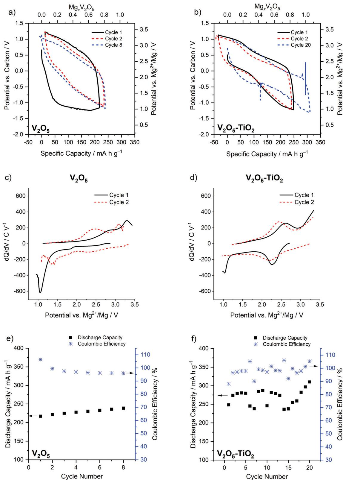
**Fig. 3** Voltage profiles of (a) the  $V_2O_5$  sample and (b) the  $V_2O_5-TiO_2$  composite;  $dQ/dV$  plots of (c) the  $V_2O_5$  sample and (d) the  $V_2O_5-TiO_2$  composite; capacity as a function of cycle number for (e) the  $V_2O_5$  sample and (f) the  $V_2O_5-TiO_2$  composite. All electrochemical measurements were performed at 110 °C.
