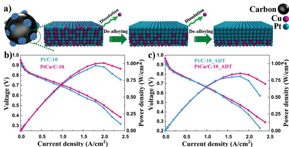
**Fig. 6** (a) Schematic image illustrating the formation of the Pt-rich shell of carbon-supported PtCu alloy catalysts. Black, blue and red spheres represent carbon, Pt and Cu, respectively. Polarization curves and power density curves of PtCu/C-10 and Pt/C-10 before (b) and after (c) ADTsc.
