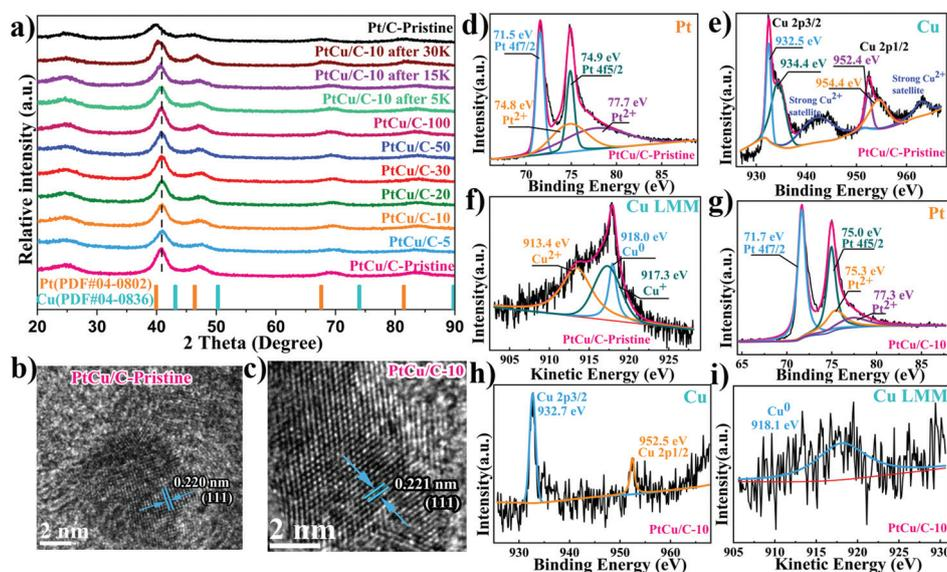
**Fig. 1** X-ray diffraction patterns of all catalysts (a). Below are peak positions of standard pure metallic Pt and Cu. HR-STEM images of PtCu/C-Pristine (b) and PtCu/C-10 (c). XPS spectra of Pt 4f, Cu 2p and Cu LM2 for PtCu/C-Pristine (d–f) and D-PtCu/C (g–i).
