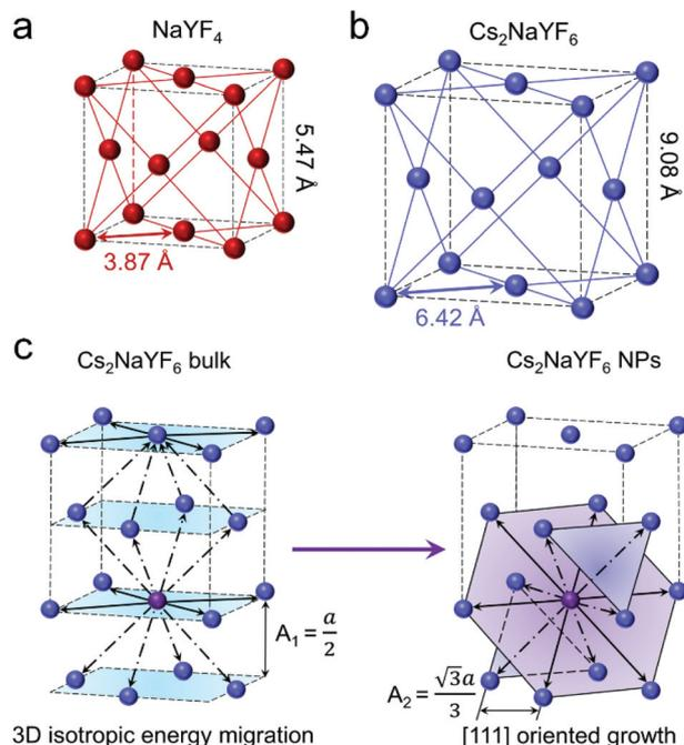
**Fig. 3** Schematic illustration of the structure of (a)  $\alpha-NaYF_4$  and (b)  $Cs_2NaYF_6:Yb/Tm$ , respectively. (c) Schematic illustration of the topological energy migration pathways in  $Cs_2NaYF_6:Yb/Tm$  bulk and NPs.
