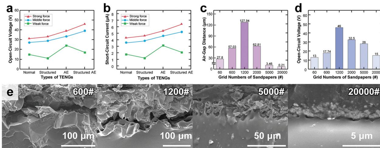
**Fig. 2** (a) The open-circuit voltage ( $V_{OC}$ ) and (b) short-circuit current ( $I_{SC}$ ) of the four types of TENGs. (c) The measured thickness of the air-gap and (d)  $V_{OC}$  with various grit numbers of commercial sandpapers. (e) The scanning electron microscope (SEM) images for the cross-section showing an air-gap between the dielectric layer and metal layer with various grit numbers of commercial sandpapers ranging from 600#, 1200#, 5000#, and 20 000#.
