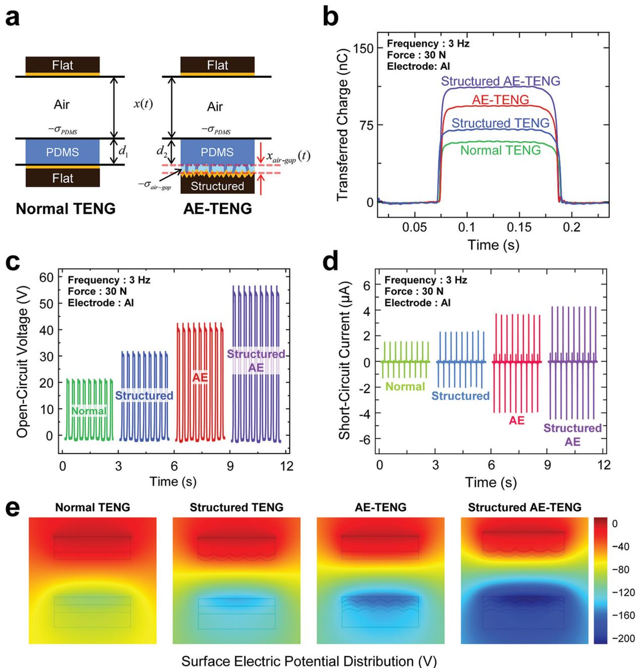
Fig. 4 (a) Schematic diagram describing the theoretical modeling for normal TENG and AE-TENG. (b) The amount of transferred charges ( $Q_{tr}$ ), (c) open-circuit voltage ( $V_{OC}$ ), and (d) short-circuit current ( $I_{SC}$ ) of the four types of TENGs at a vibration frequency of 3 Hz and an applied force of 30 N. (e) The visualization of the electric potential distribution of the four types of TENGs simulated by using a simulation software.
