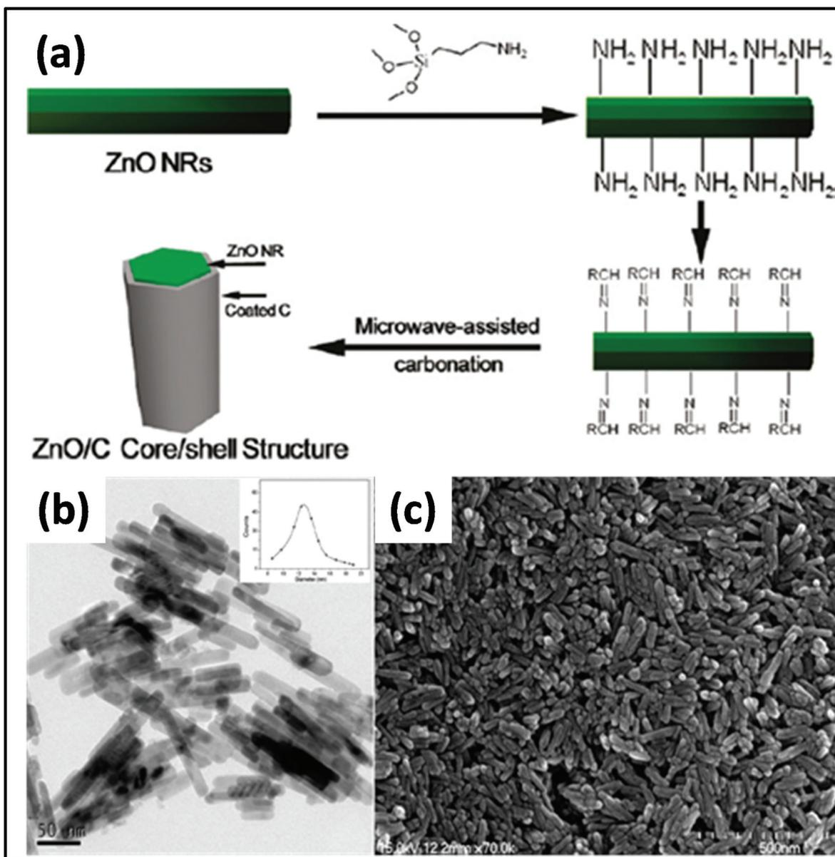
Fig. 10 (a) Schematic diagram showing the synthesis of carbon-coated ZnO. (b) TEM (inset: average size distribution of 200 rods) and (c) SEM images of ZnO nanorods.<sup>204</sup> Reprinted (adapted) with permission from ref. 204, copyright (2009), the American Chemical Society.
