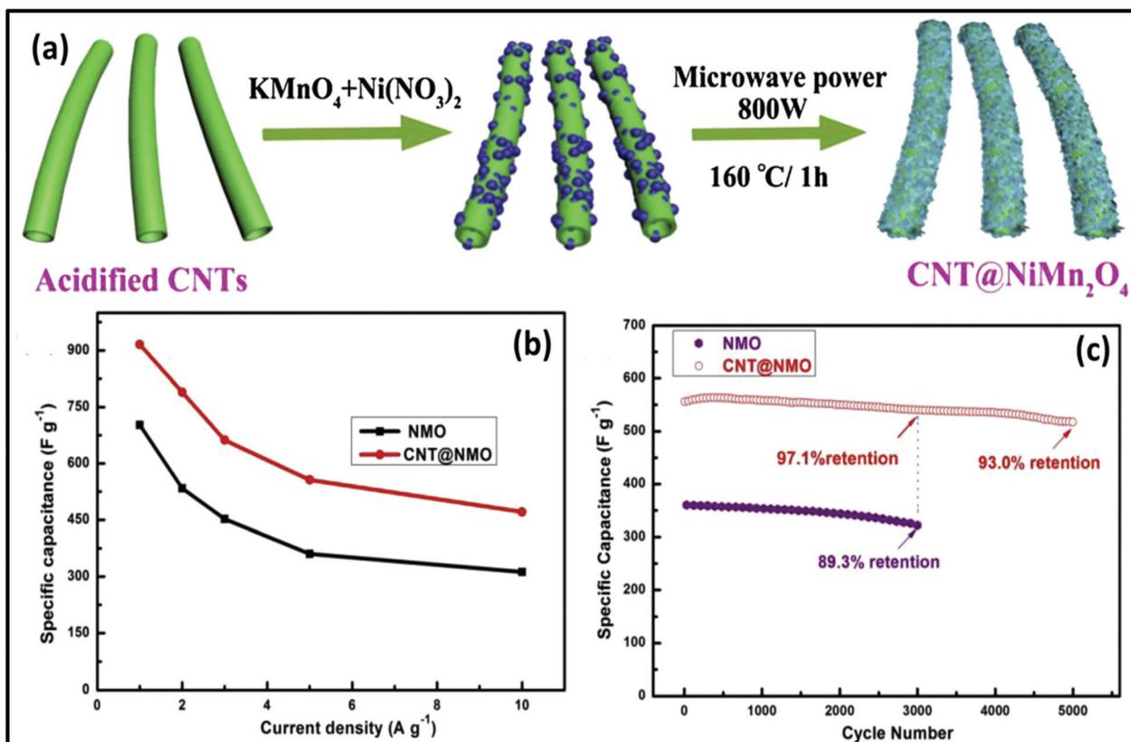
Fig. 19 (a) Schematic representation of the formation of CNT@NiMn<sub>2</sub>O<sub>4</sub> nanocomposite, (b) specific capacitance of NiMn<sub>2</sub>O<sub>4</sub> and CNT@NiMn<sub>2</sub>O<sub>4</sub> nanocomposite at different current densities and (c) cycling stability of NiMn<sub>2</sub>O<sub>4</sub> and CNT@NiMn<sub>2</sub>O<sub>4</sub> nanocomposite at 5  $\text{A g}^{-1}$ . Reprinted (adapted) with permission from ref. 273, copyright (2020), Elsevier B.V. All rights reserved.
