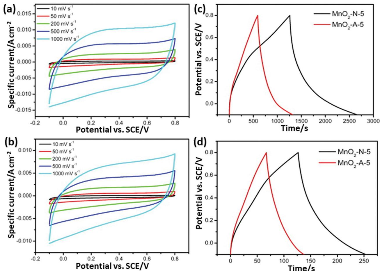
Fig. 16 (a and b) CV curves of MnO<sub>2</sub>-N-5 and MnO<sub>2</sub>-A-5 at different scan rates and (c and d) charge/discharge curves of MnO<sub>2</sub>-N-5 and MnO<sub>2</sub>-A-5 at current densities of 0.2 A g<sup>-1</sup> and 1 A g<sup>-1</sup>, respectively.<sup>257</sup> Reprinted (adapted) with permission from ref. 257, copyright (2013), Elsevier B.V. All rights reserved.
