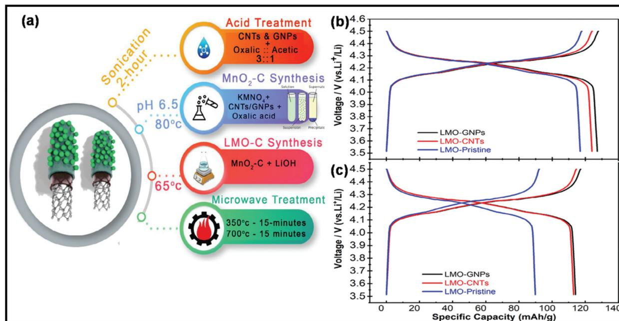
**Fig. 23** (a) Schematic of the experimental details for the synthesis of LiMn<sub>2</sub>O<sub>4</sub>/CNT/GNP nanocomposite. (b) Galvanostatic charge/discharge behavior of LiMn<sub>2</sub>O<sub>4</sub>/GNPs, LiMn<sub>2</sub>O<sub>4</sub>-CNTs and pristine LiMn<sub>2</sub>O<sub>4</sub> at 0.1 C and 25 °C (b) 1st cycle and (c) 50th cycle.<sup>322</sup> Reprinted (adapted) with permission from ref. 322, copyright (2021), Wiley, All rights reserved.
