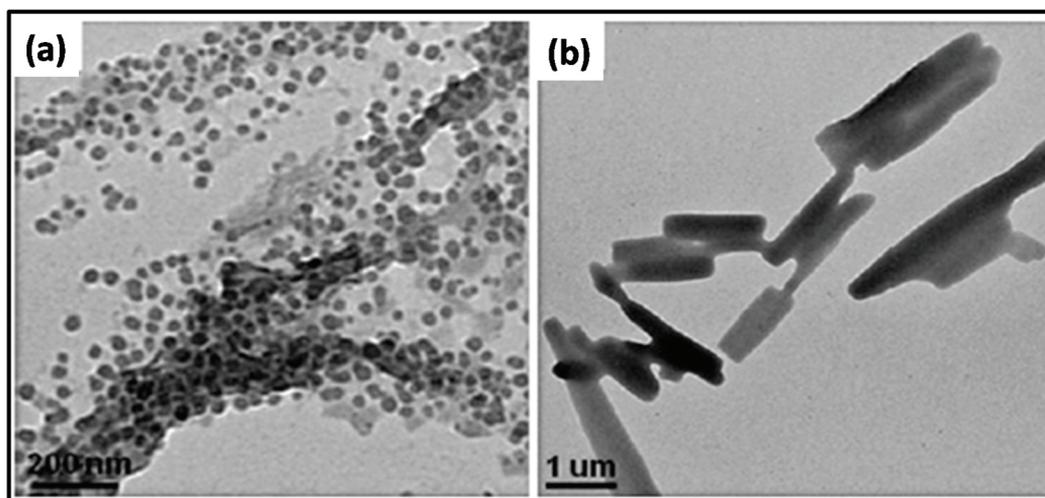
**Fig. 7** TEM images of ZnO nanostructures prepared by MWI of 0.1 M zinc acetate solution in pure oleic acid for 30 s (a) and 60 s (b).<sup>161</sup> Reprinted (adapted) with permission from ref. 161, copyright (2013), Springer. All rights reserved.
