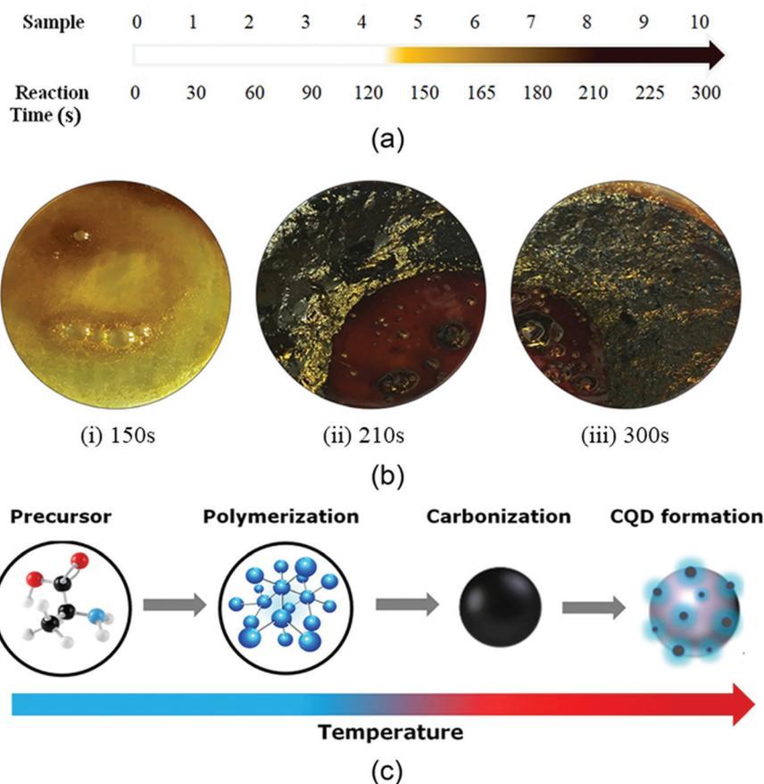
**Fig. 11** (a) Change in sample color with reaction time. (b) Samples depicting the change in color and CQD formation upon heat treatment of (i) 150 s, (ii) 210 s, and (iii) 300 s. (c) Reaction pathway for the synthesis of CQDs with an increase in temperature.<sup>208</sup> Reprinted (adapted) with permission from ref. 208, copyright (2020), Taylor & Francis Group. All rights reserved.
