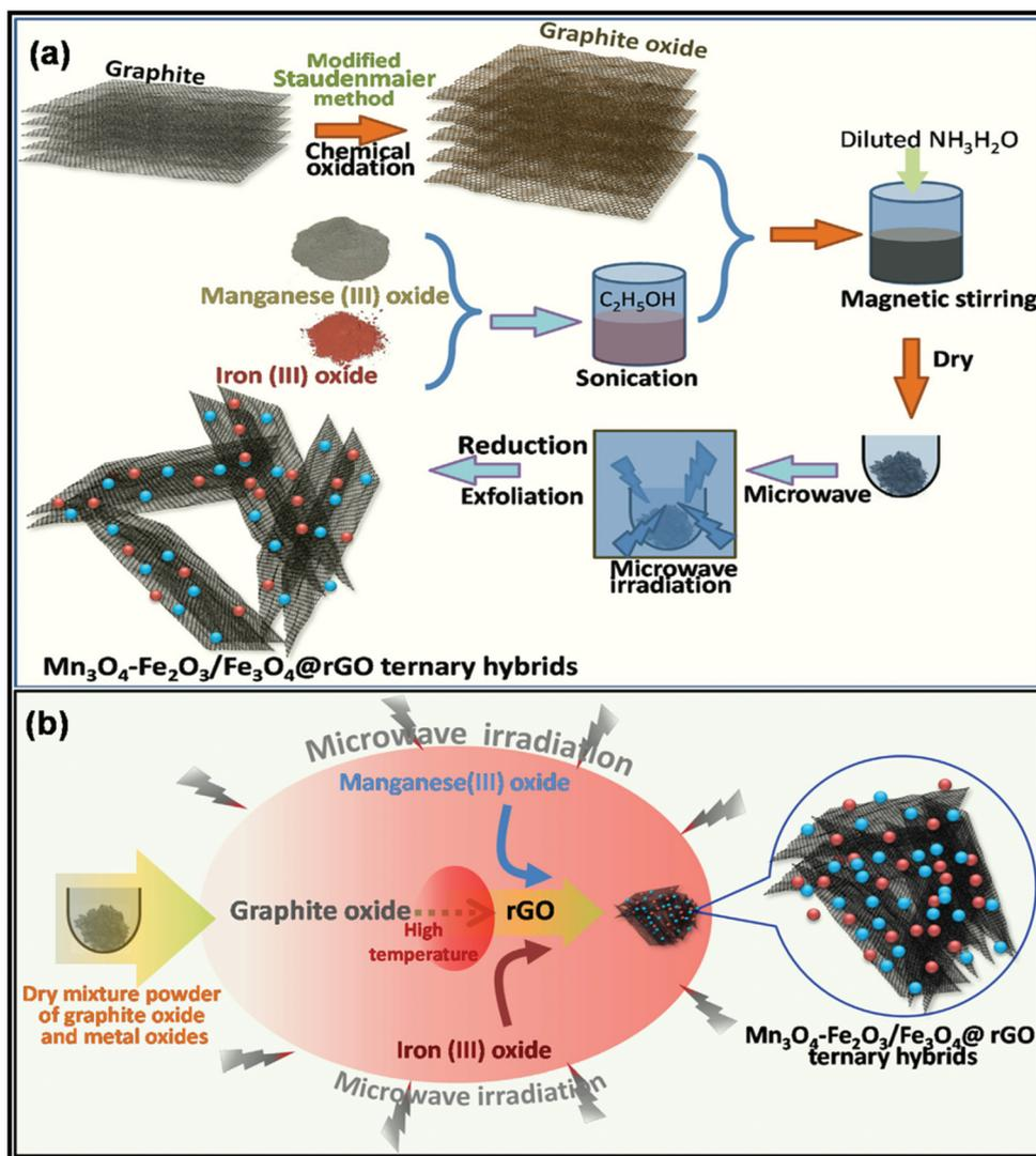
Fig. 13 Schematic presentation of the (a) synthesis process and (b) mechanism of MW-assisted formation of Mn<sub>3</sub>O<sub>4</sub>-Fe<sub>2</sub>O<sub>3</sub>/Fe<sub>3</sub>O<sub>4</sub>@rGO ternary hybrid.<sup>222</sup> Reprinted (adapted) with permission from ref. 222, copyright (2020), Elsevier B.V. All rights reserved.
