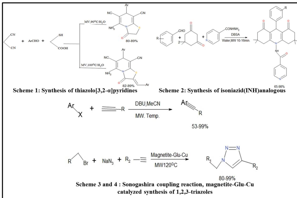
Fig. 14 Scheme for synthesis via the MW-assisted method.<sup>76,250–252</sup>
