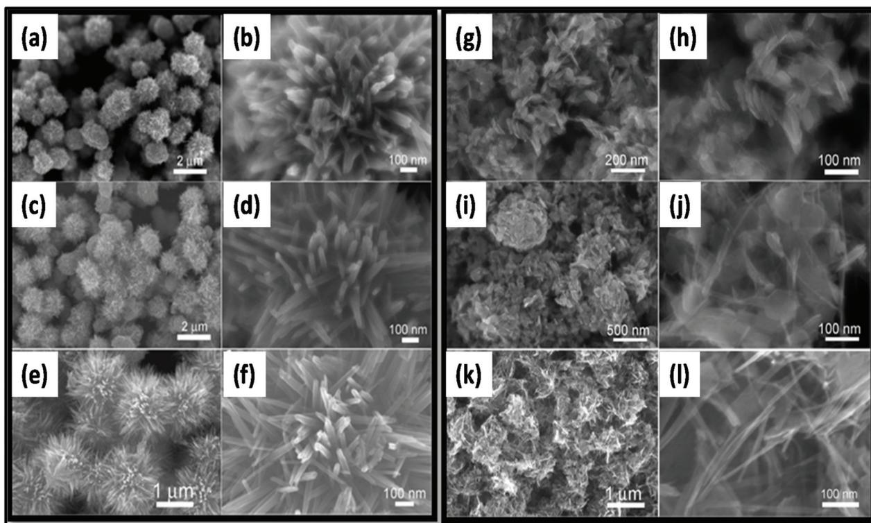
Fig. 15 SEM images of MnO<sub>2</sub> prepared at (a, b, g, and h) 5 min, (c, d, i, and j) 10 min, and (e, f, k, and l) 30 min under (a–f) acidic condition and (g–l) neutral condition.<sup>257</sup> Reprinted (adapted) with permission from ref. 257, copyright (2013), Elsevier B.V. All rights reserved.
