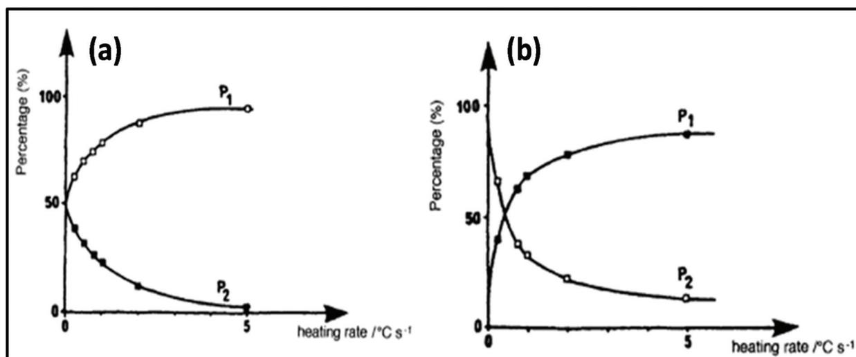
Fig. 5 Controlling rate of reaction using MW heating: (a) induced heating and (b) inversion heating.<sup>113</sup> Reprinted (adapted) with permission from ref. 113, copyright (1993), Elsevier B.V. All rights reserved.
