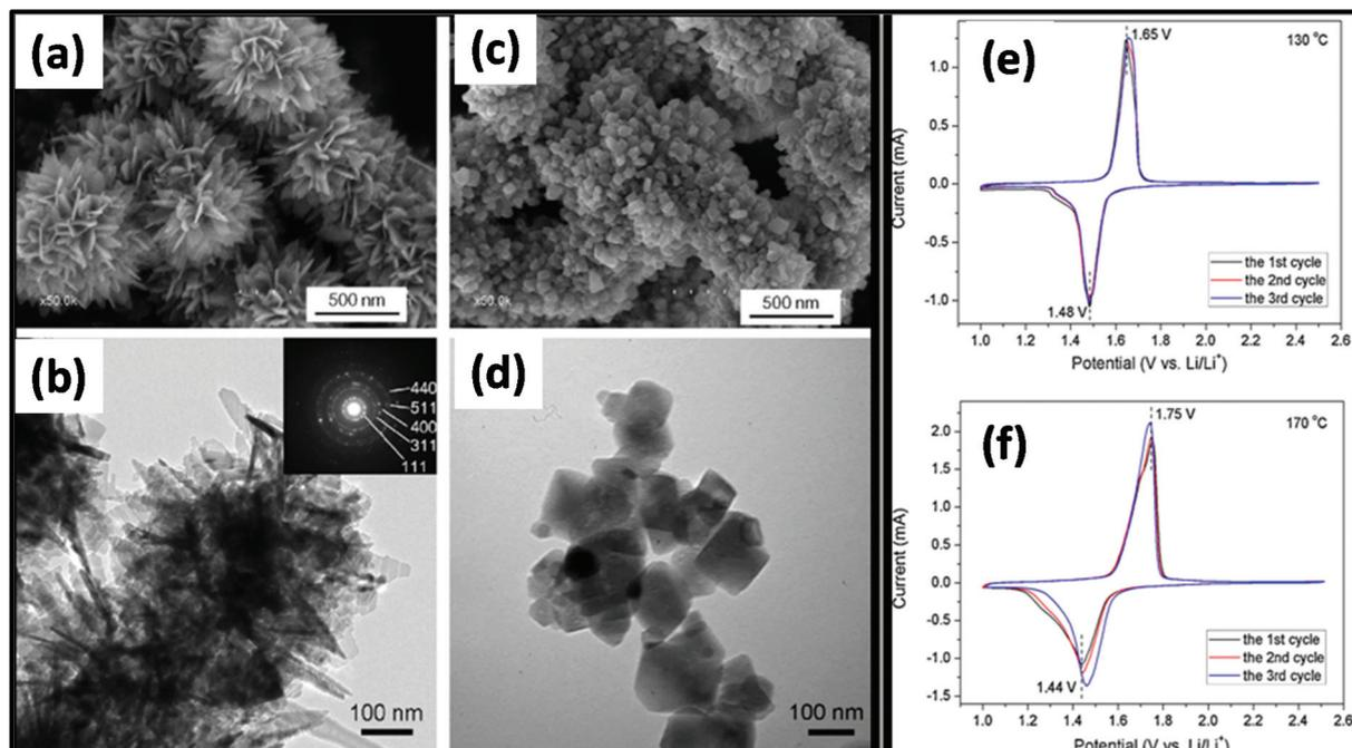
Fig. 20 (a and c) SEM images of  $\text{Li}_4\text{Ti}_5\text{O}_{12}$  synthesized at 130 °C and (b and d) TEM images of  $\text{Li}_4\text{Ti}_5\text{O}_{12}$  synthesized at 170 °C. (e and f) CV curves of  $\text{Li}_4\text{Ti}_5\text{O}_{12}$  prepared at (e) 130 °C and (f) 170 °C in the first three cycles at a scan rate of 0.2  $\text{mV s}^{-1}$ . Reprinted (adapted) with permission from ref. 281, copyright (2012), Elsevier B.V. All rights reserved.
