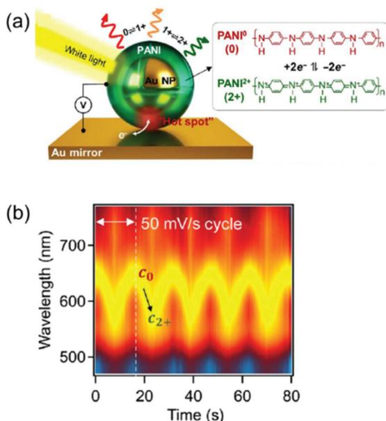
**Fig. 8** (a) Schematic representation of eNPoM geometry, which changes the redox states of PANI in hot spot under electrochemical potential. (b) Time-dependent normalized DF scattering spectra of a single spot in eNPoM showed dramatic and reversible tuning by the redox states of PANI. Reprinted with permission.<sup>26</sup> Copyright 2019 American Association for the Advancement of Science.
