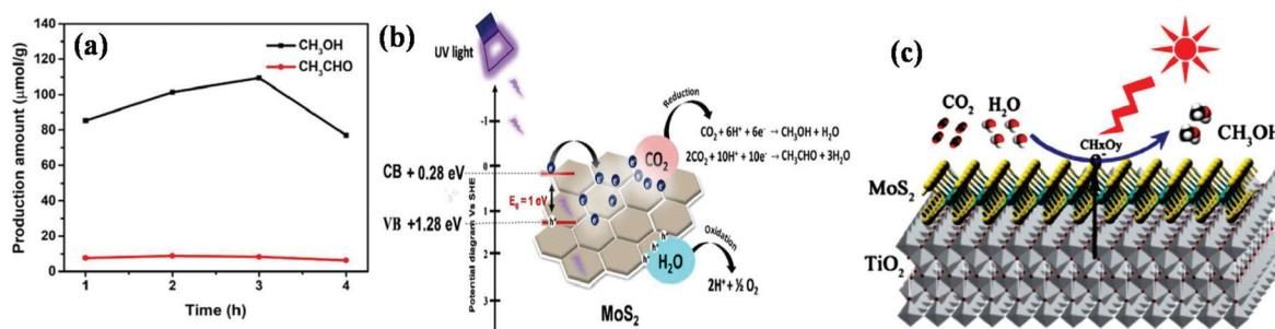
**Fig. 14** (a) Rate of  $\text{CO}_2$  reduction by  $\text{MoS}_2$  sheets in 0.5 M  $\text{NaHCO}_3$  and (b) schematic representation of the mechanistic pathway for photocatalytic  $\text{CO}_2$  reduction over  $\text{MoS}_2$  sheets. Reproduced with permission.<sup>173</sup> (c) Schematic illustration of the photoreduction of  $\text{CO}_2$  to  $\text{CH}_3\text{OH}$  in the  $\text{MoS}_2/\text{TiO}_2$  heterostructure. Reproduced with permission.<sup>170</sup>
