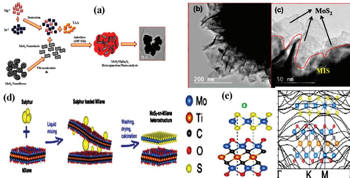
Fig. 6 (a) Schematic diagram showing the growth mechanism and (b) and (c) corresponding HRTEM images of  $\text{MoS}_2/\text{MgIn}_2\text{S}_4$  heterojunction photocatalyst. Reproduced with permission.<sup>90</sup> (d) Schematic representation of the fabrication of  $\text{MoS}_2/\text{MXene}$  hybrids and (e) structural stacking patterns and electronic band structure of  $\text{MoS}_2/\text{Mo}_2\text{TiC}_2\text{O}_4$ . Reproduced with permission.<sup>105</sup>
