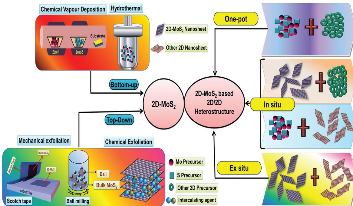
**Scheme 2** Schematic illustration of the various techniques used for the synthesis of 2D-MoS<sub>2</sub> and its 2D/2D-heterostructures.
