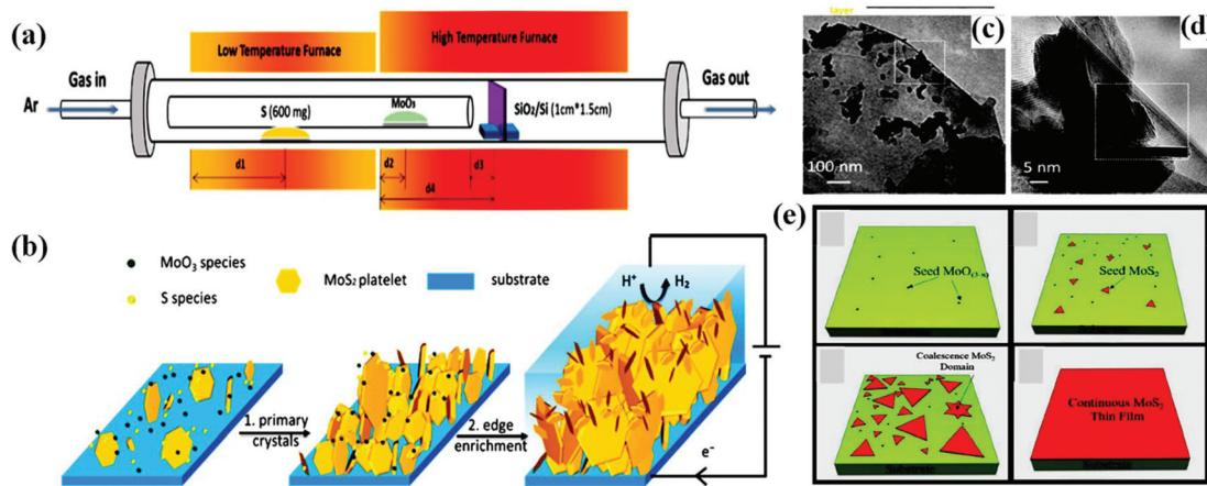
**Fig. 3** (a) Schematic representation showing the experimental CVD setup, (b) mechanistic demonstration of the edge enrichment of MoS<sub>2</sub>, (c) and (d) TEM images of the petal site showing the nucleation of vertically aligned nanoflakes on the top-layer crystals. Reproduced from ref. 85. (e) Schematic illustration of monolayer MoS<sub>2</sub> growth on a Piranha-treated substrate. Reproduced from ref. 86.
