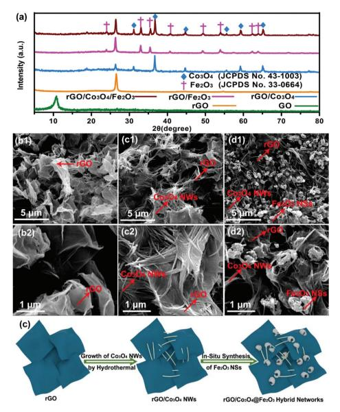
Fig. 1 (a) XRD results of GO,  $rGO/Co_3O_4$  NWs,  $rGO/Fe_2O_3$  NSs and  $rGO/Co_3O_4$ @Fe $_2O_3$  hybrid networks. SEM images of GO (b1-b2),  $rGO/Co_3O_4$  (c1-c2) and  $rGO/Co_3O_4$ @Fe $_2O_3$  (d1-d2). The insets in b2, c2 and d2 are the schematic diagrams of the corresponding morphologies. (c) Schematic of the formation for  $rGO/Co_3O_4$ @Fe $_2O_3$  hybrid networks.
