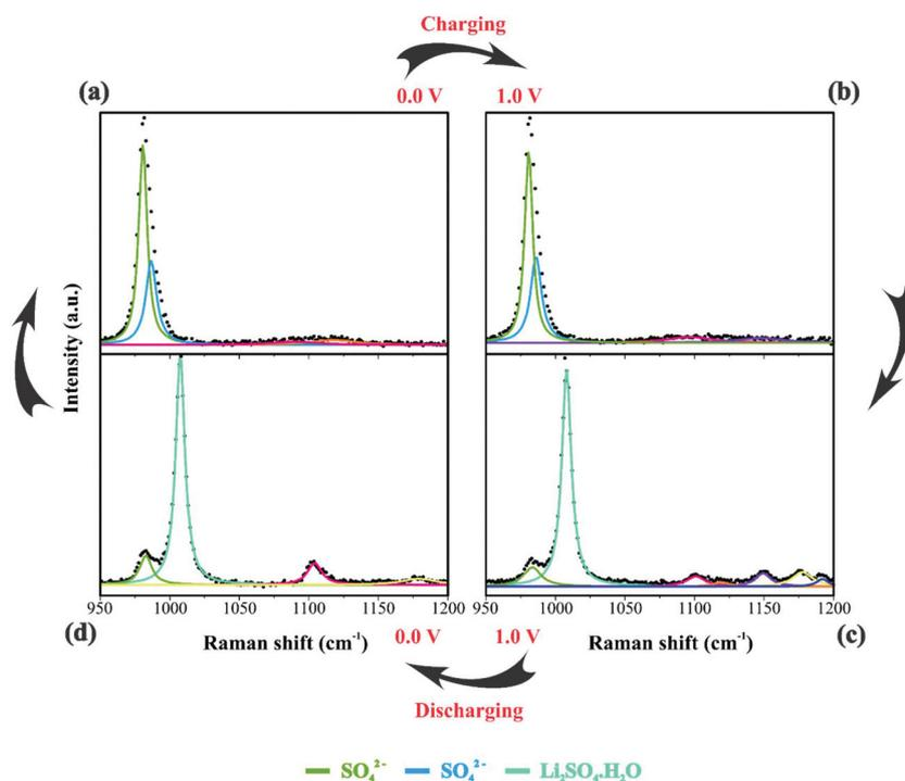
Fig. 5 Raman spectra of the electrode/electrolyte interface under cyclic voltammetry at scan rate  $0.15 \text{ mV s}^{-1}$  from (a) 0 V to (b) 1 V during charge and from (c) 1 V to (d) 0 V during discharge. Spectra intensities are normalized from 0 to 1 in the  $950$  to  $1200 \text{ cm}^{-1}$ . Electrodes were housed in an EI Cell filled with  $80 \mu\text{L}$  of a  $1.0 \text{ M Li}_2\text{SO}_4$  aqueous solution.
