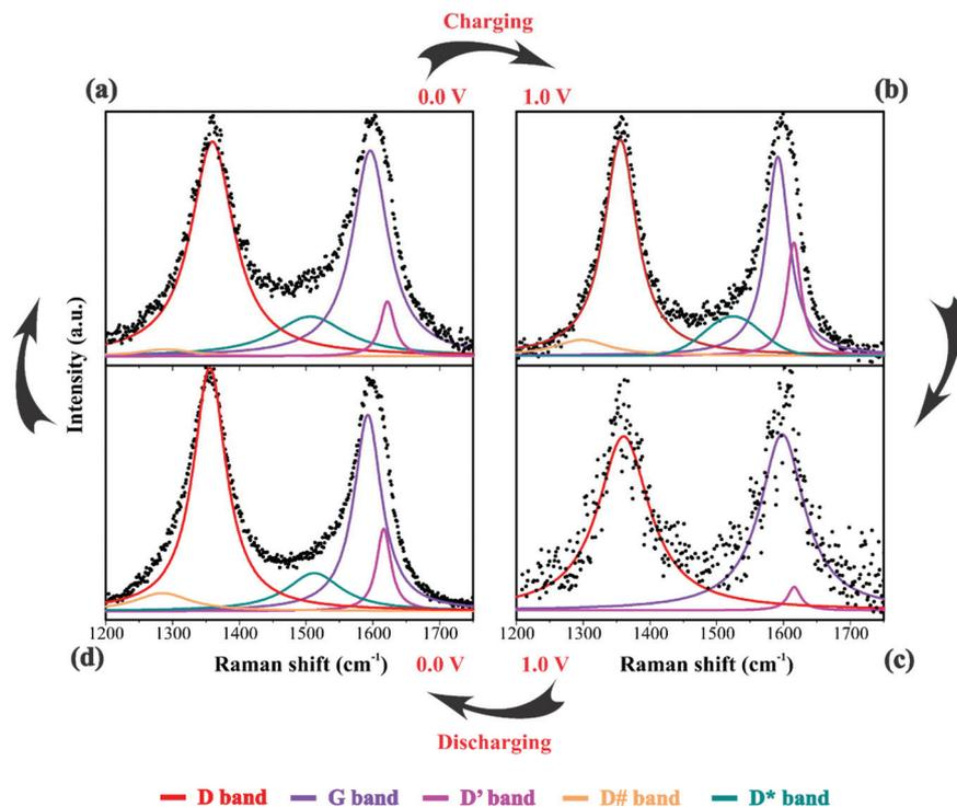
**Fig. 6** Raman spectra of the electrode/electrolyte interface under cyclic voltammetry at scan rate  $0.15 \text{ mV s}^{-1}$  from (a) 0 V to (b) 1 V during charge and from (c) 1 V to (d) 0 V during discharge. Spectra intensities are normalized from 0 to 1 in the  $1200$  to  $1750 \text{ cm}^{-1}$ . Electrodes were housed in an EL Cell filled with  $80 \mu\text{L}$  of a  $1 \text{ M Li}_2\text{SO}_4$  aqueous solution. Deconvolution considered five bands as described in Fig. 1(d).
