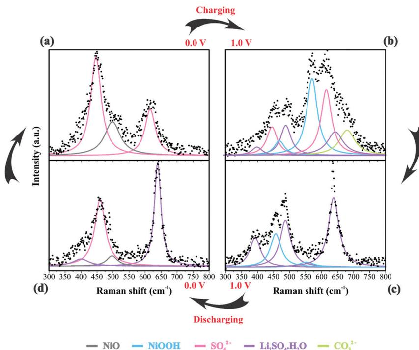
Fig. 4 Raman spectra of the electrode/electrolyte interface under cyclic voltammetry at a scan rate of  $0.15 \text{ mV s}^{-1}$  from (a) 0 to (b) 1 V during charge and from (c) 1 V to (d) 0 V during discharge. Spectra intensities are normalized from 0 to 1 in the  $300$  to  $800 \text{ cm}^{-1}$ . Working electrodes were housed in a symmetrical EI Cell filled with  $80 \mu\text{L}$  of a  $1 \text{ M Li}_2\text{SO}_4$  aqueous solution.
