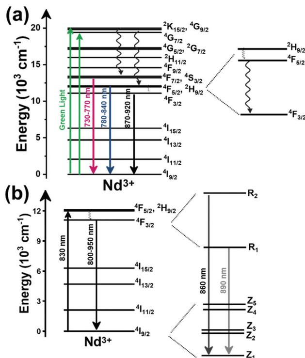
Fig. 11 Mechanisms of generation of the emission bands in single  $\text{Nd}^{3+}$ -doped nanoparticles after being excited with: (a) a green light source (the magnification detail depicts the thermally coupled  ${}^4\text{F}_{5/2}$  and  ${}^4\text{F}_{3/2}$  levels), and (b) a near infrared light source.
