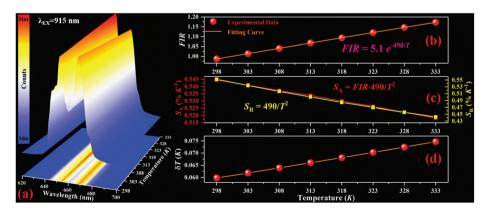
Fig. 4 (a) Red UC emission normalized at 669 nm, (b) FIR, (c) absolute sensitivity  $S_A$  and relative sensitivity  $S_R$  and (d) temperature resolution  $\delta T_G$  as a function of temperature in NYEM@NaScF4@SiO2@Cu2S.
