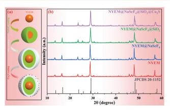
Fig. 1 (a) A description of the preparation of NYEM@NaScF $_4$ @SiO $_2$ @Cu $_2$ S. (b) XRD diffraction patterns of the samples synthesized at various steps along with the reference data of hexagonal NaScF $_4$  (JCPDS 20-1152).
