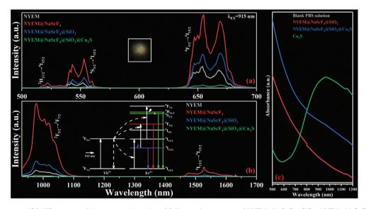
Fig. 3 (a) UC spectra and (b) NIR spectra of the prepared samples. (c) Absorption spectra of NYEM@NaScF4@SiO<sub>2</sub>@Cu<sub>2</sub>S and Cu<sub>2</sub>S dispersed in PBS solution as well as the blank PBS solution. The inset in (a) is the digital photo of NYEM@NaScF<sub>4</sub>@SiO<sub>2</sub>@Cu<sub>2</sub>S excited by 915 nm wavelength. The inset in (b) is the ET processes between Yb<sup>3+</sup> and Er<sup>3+</sup>.
