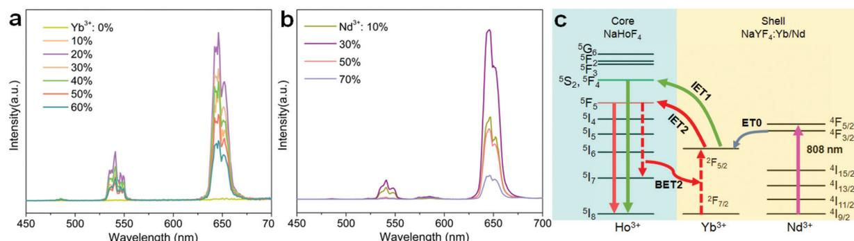
Fig. 5 (a and b) Upconversion emission spectra of  $\text{NaHoF}_4@\text{NaYF}_4:\text{Yb}(0\text{--}60 \text{ mol}\%)$  and  $\text{NaHoF}_4@\text{NaYF}_4:\text{Yb}(20 \text{ mol}\%)@\text{Nd}(10\text{--}70 \text{ mol}\%)$  core–shell nanoparticles under 980 and 808 nm excitations, respectively. (c) Schematic of the energy transport processes in the  $\text{Nd}^{3+}$ -sensitized upconversion system.
