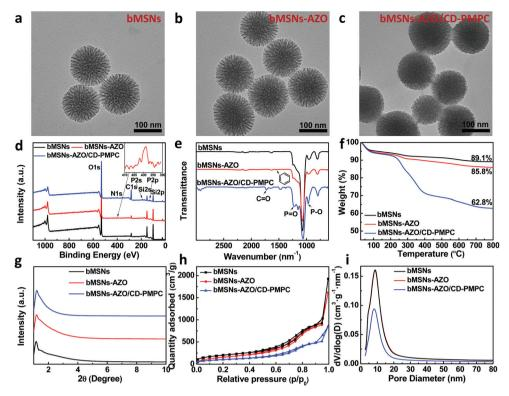
Fig. 2 Characterizations of the nanoparticles. TEM images of bMSNs (a), bMSNs-AZO (b) and bMSNs-AZO/CD-PMPC (c). XPS spectra (d), FTIR spectra (e), TGA curves (f), small-angle XRD patterns (g), N<sub>2</sub> adsorption-desorption isotherms (h) and the pore size distribution (i) of bMSNs, bMSNs-AZO and bMSNs-AZO/CD-PMPC.
