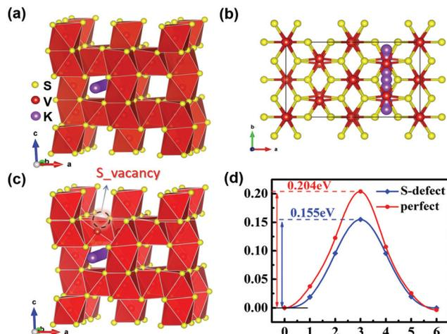
Fig. 7 The minimum energy path for the K atom diffusion pathways in (a and b) P- $V_5S_8$  and (c) S-defective  $V_5S_8$ .<sup>17</sup> (d) The corresponding barrier energy. The yellow, red and purple balls represent the S, V and K atoms, respectively.
