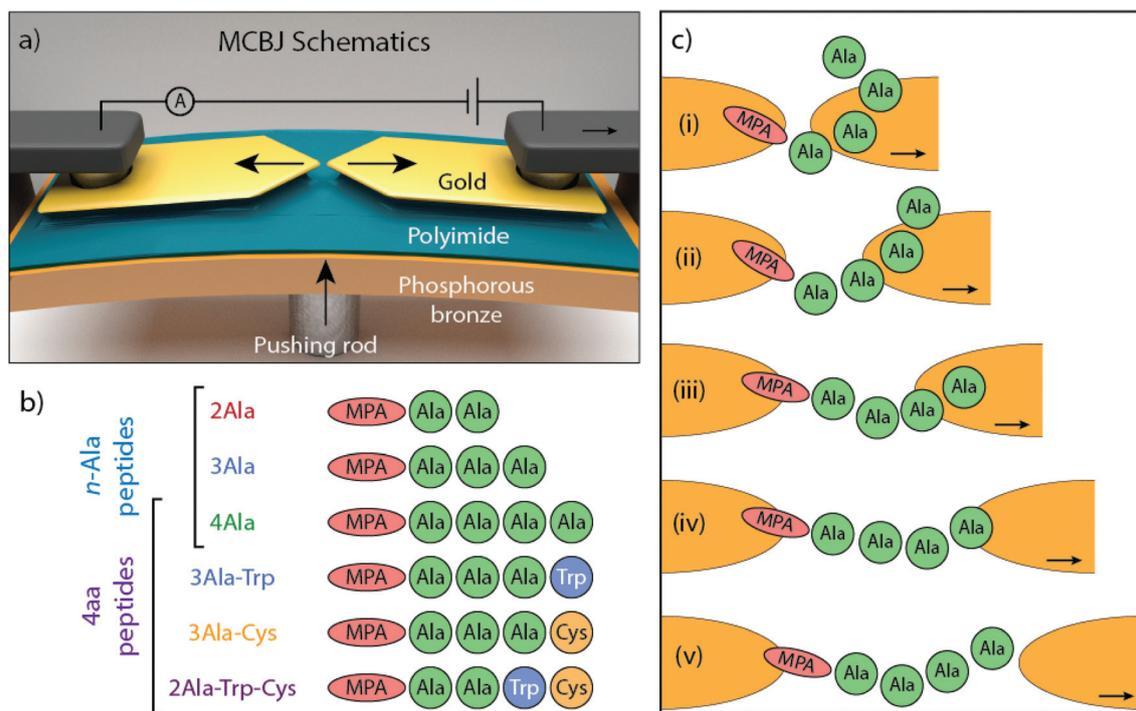
**Fig. 1** (a) Schematic representation of the Mechanically Controlled Break-Junction (MCBJ) setup. (b) Schematic representation of the structure of the peptides measured in this work. (c) Cartoon representation of possible conformations during a breaking event with 4Ala: the peptide is anchored to one of the gold electrodes *via* the MPA linker group and it forms various metastable configurations as it is dragged across the junction.
