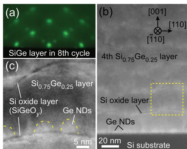
**Fig. 2** (a) RHEED pattern of the  $\text{Si}_{0.75}\text{Ge}_{0.25}$  layer in the 8th cycle structure of the Ge ND ( $\sim 8$  nm)/ $\text{Si}_{0.75}\text{Ge}_{0.25}$  ( $\sim 22$  nm) film. (b and c) Cross-sectional ADF-TEM images of the Ge ND ( $\sim 8$  nm)/ $\text{Si}_{0.75}\text{Ge}_{0.25}$  ( $\sim 22$  nm) film: (b) low and high (c) magnifications. The image in (c) corresponds to the region marked by the dotted square in (b).
