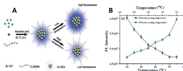
**Fig. 25** (A) Schematic illustration of the formation mechanism of CuNCs with temperature-dependent fluorescence. Republished with permission from ref. 134. Copyright 2014 Royal Society of Chemistry. (B) PL reversibility exhibited by the HSA-CuNCs as a function of temperature. Reprinted with permission from ref. 50. Copyright 2015 American Chemical Society.
