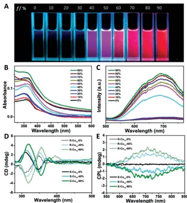
**Fig. 24** (A) Photographs of fluorescent  $R\text{-Cu}_{14}$  in solutions with different fractions of *n*-hexane. (B) UV/Vis absorption spectra, (C) emission spectra, (D) CD spectra, and (E) CPL spectra of  $R/S\text{-Cu}_{14}$  in DCM/*n*-hexane mixtures with different (*f*) values. Adapted with permission from ref. 173. Copyright 2019 Wiley-VCH Verlag GmbH & Co. KGaA, Weinheim.
