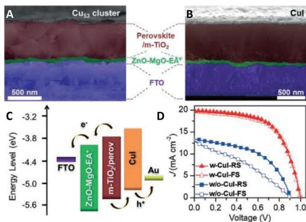
**Fig. 38** Device structure and cross-sectional SEM image of (A)  $\text{Cu}_{53}$  and (B)  $\text{CuI}$  on perovskite films. (C) Energy-level diagram of  $\text{CuI}$ -based perovskite solar cell (PSC). (D) Best  $J$ - $V$  curves of devices with  $\text{CuI}$  (w- $\text{CuI}$ ) and without  $\text{CuI}$  (w/o- $\text{CuI}$ ). FS = forward scan, RS = reverse scan. Adapted with permission from ref. 194. Copyright 2019 Wiley-VCH Verlag GmbH & Co. KGaA, Weinheim.
