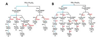
Theoretical reaction schemes for CO<sub>2</sub> electroreduction on [Cu<sub>32</sub>H<sub>20</sub>{S<sub>2</sub>P(O<sup>i</sup>Pr)<sub>2</sub>}<sub>12</sub>] to form (A) HCOOH and (B) CO via six different pathways as described in ref. 188 (Reprinted with permission, Copyright 2017 American Chemical Society). The calculated free energy difference  $(\Delta G)$  for each elementary step is shown under each intermediate state. The most favourable reaction pathway is highlighted in blue.
