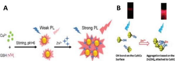
**Fig. 21** (A) Schematic illustration of the preparation of GSH-capped CuNCs and the aggregation-induced PL enhancement of CuNCs in the presence of Zn<sup>2+</sup>. Reprinted with permission from ref. 225. Copyright 2017 Elsevier. (B) Scheme for the mechanism of the aggregation-induced fluorescence enhancement for CuNCs in the presence of Zn<sup>2+</sup>. Republished with permission from ref. 110. Copyright 2016 Royal Society of Chemistry.
