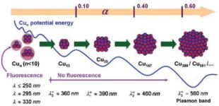
Fig. 5 Schematic representation of copper nanocluster size evolution with increasing the molar percentage (a) of NaBH<sub>4</sub>. The clusters with  $n \le 13$  are fluorescent, whereas big particles with  $n \ge 309$  show characteristic plasmon resonance band. Reprinted with permission from ref. 101. Copyright 2009 American Chemical Society.
