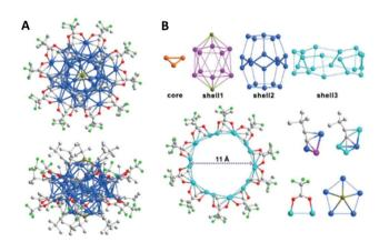
Fig. 14 (A) Molecular structure of a  $Cu_{53}$  cluster: the view along an approximately five-fold axis (top), and general view (bottom). Colour codes: Cu; blue, F; light green, Cl; dark yellow, O; red, C; grey. Hydrogen atoms are omitted for clarity. (B) Shell-by-shell structural analyses of the cluster framework. Adapted with permission from ref. 194. Copyright 2019 Wiley-VCH Verlag GmbH & Co. KGaA, Weinheim.
