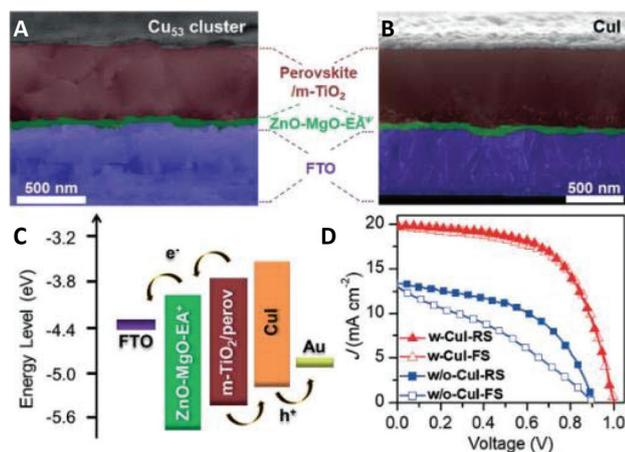
**Fig. 38** Device structure and cross-sectional SEM image of (A)  $\text{Cu}_{53}$  and (B) CuI on perovskite films. (C) Energy-level diagram of CuI-based perovskite solar cell (PSC). (D) Best  $J$ - $V$  curves of devices with CuI (w-CuI) and without CuI (w/o-CuI). FS = forward scan, RS = reverse scan. Adapted with permission from ref. 194. Copyright 2019 Wiley-VCH Verlag GmbH & Co. KGaA, Weinheim.
