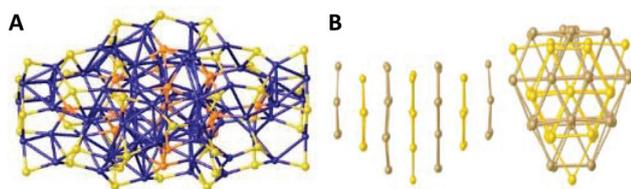
**Fig. 10** (A) The core structure of the  $\text{Cu}_{74}\text{S}_{15}(\text{2-PET})_{45}$  cluster. Bridged-sulphur atoms are in orange, and sulphur atoms belonging to ligands are in yellow. The layers are labelled as L1 to L7 from left to right. (B) Side and top views of the layer organization of the sulphur atoms. Two types of layers (A in yellow, B in gold) organize themselves in an A-B-A pattern. Reprinted with permission from ref. 195. Copyright 2020 American Chemical Society.
