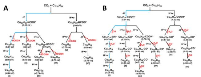
Scheme 9 Theoretical reaction schemes for  $\text{CO}_2$  electroreduction on  $[\text{Cu}_{32}\text{H}_{20}\{\text{S}_2\text{P}(\text{O}^i\text{Pr})_2\}_{12}]$  to form (A) HCOOH and (B) CO via six different pathways as described in ref. 188 (Reprinted with permission, Copyright 2017 American Chemical Society). The calculated free energy difference ( $\Delta G$ ) for each elementary step is shown under each intermediate state. The most favourable reaction pathway is highlighted in blue.
