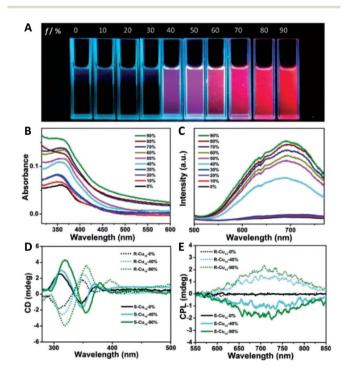
Fig. 24 (A) Photographs of fluorescent R-Cu<sub>14</sub> in solutions with different fractions of *n*-hexane. (B) UV/Vis absorption spectra, (C) emission spectra, (D) CD spectra, and (E) CPL spectra of R/S-Cu<sub>14</sub> in DCM/ n-hexane mixtures with different (fv) values. Adapted with permission from ref. 173. Copyright 2019 Wiley-VCH Verlag GmbH & Co. KGaA,
