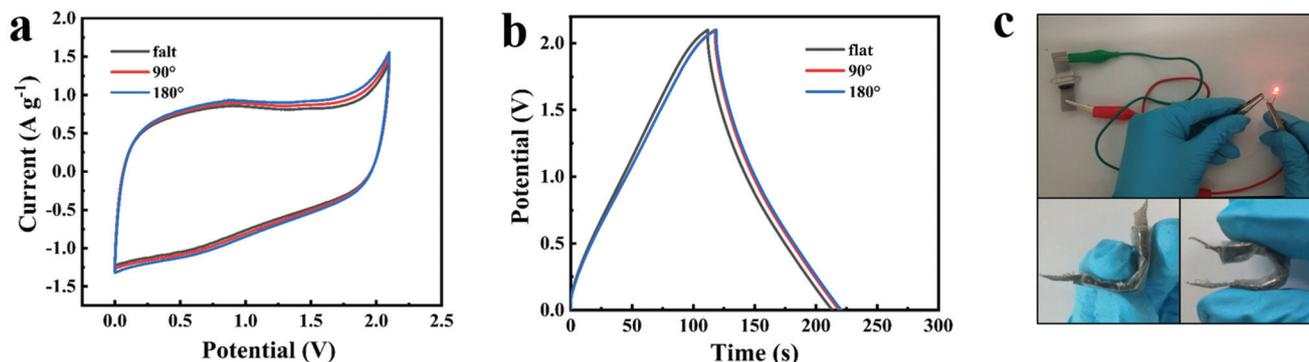
Fig. 6 CV curves at  $10 \text{ mV s}^{-1}$  (a) and GCD profiles at  $1 \text{ A g}^{-1}$  (b) of the assembled flexible device at  $0$ – $180^\circ$ . Optical images of the flexible device under different bending conditions (c).
