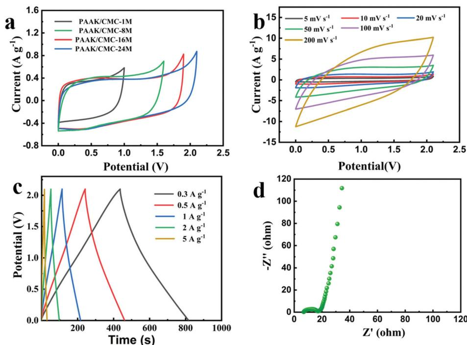
Fig. 3 Voltage windows of PAAK/CMC-1, 8, 16, 24 M at  $5 \text{ mV s}^{-1}$  (a), CV curves from  $5 \text{ mV s}^{-1}$  to  $200 \text{ mV s}^{-1}$  (b), GCD profiles from  $0.3 \text{ A g}^{-1}$  to  $5 \text{ A g}^{-1}$  (c) and EIS (d) of the NG//NG quasi-solid-state supercapacitor with the PAAK/CMC-24 M polyelectrolyte hydrogel.
