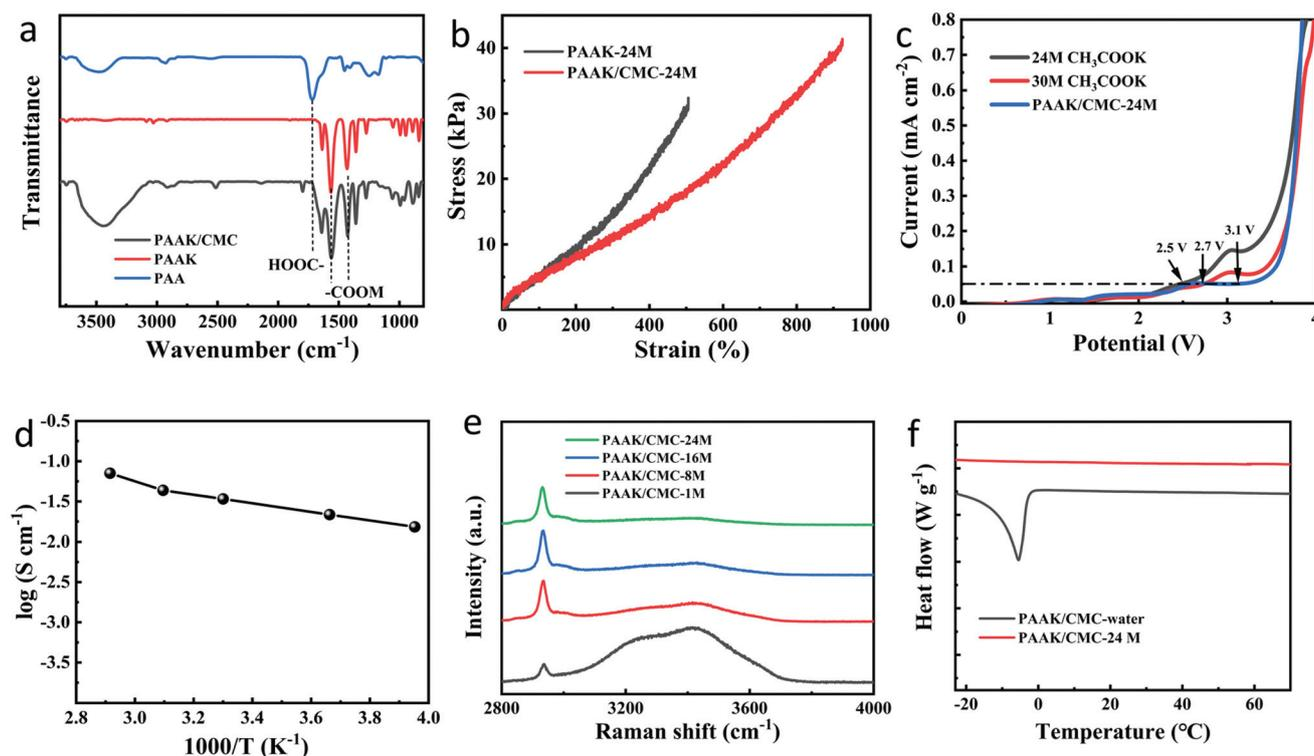
Fig. 2 FTIR spectra of pure PAA, PAAK and PAAK/CMC hydrogel (a), stress–strain curves of PAAK-24 M and PAAK/CMC-24 M (b), LSV curves at a scan rate of  $10 \text{ mV s}^{-1}$  (c), ionic conductivity of the PAAK/CMC-24 M at a temperature from  $-20$  to  $70$  °C (d), Raman spectra of PAAK/CMC-x (e). DSC thermograms of pure water and 24 M  $\text{CH}_3\text{COOK}$  in the PAAK/CMC hydrogel (f).
