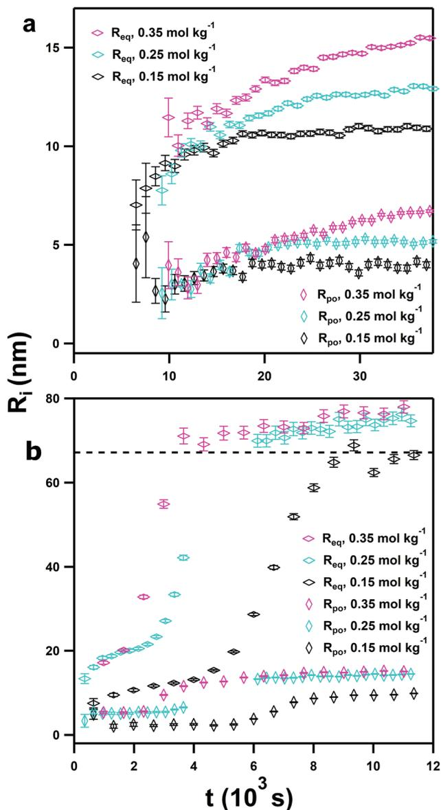
**Fig. 5** (a) Fitted equatorial ( $R_{eq}$ ) and polar ( $R_{po}$ ) radii as a function of time for the pure DES and (b) for the hydrated DES, in the H : D contrast. The tie line for (b) is drawn at 65.5 nm, the approximate length scale maximum. Above this length the model fit is no longer sensitive to changes in this parameter, when using model-based (oblate-ellipsoid) fitting to the data within SasView.
