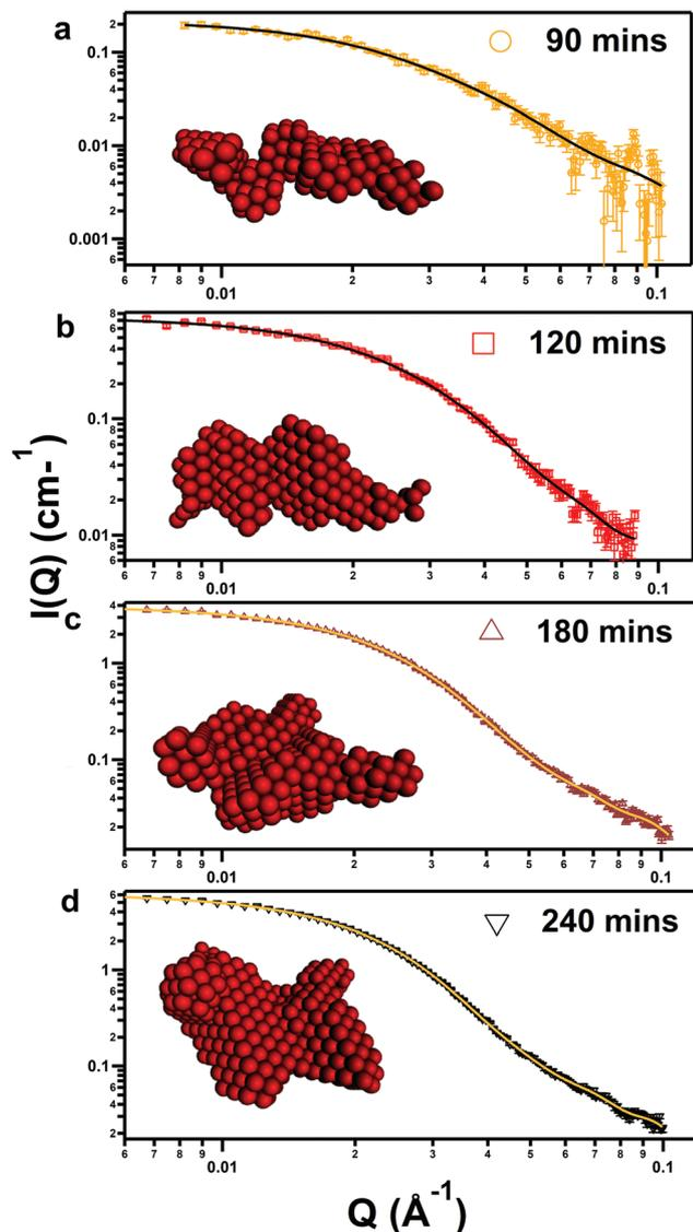
**Fig. 6** SAXS data of iron oxide (markers) corresponding with pure DES samples containing  $0.25 \text{ mol kg}^{-1}$  of iron, reacted in an oven at  $90^\circ \text{C}$  for (a) 90 min (5400 s), (b) 120 min (7200 s), (c) 180 min (10 800 s), (d) 240 min (14 400 s). Fits to the data (lines) use software from the ATSAS package,<sup>59</sup> which determines the overall nanoparticle shapes (inset) by simulated monophase annealing of dummy atoms.
