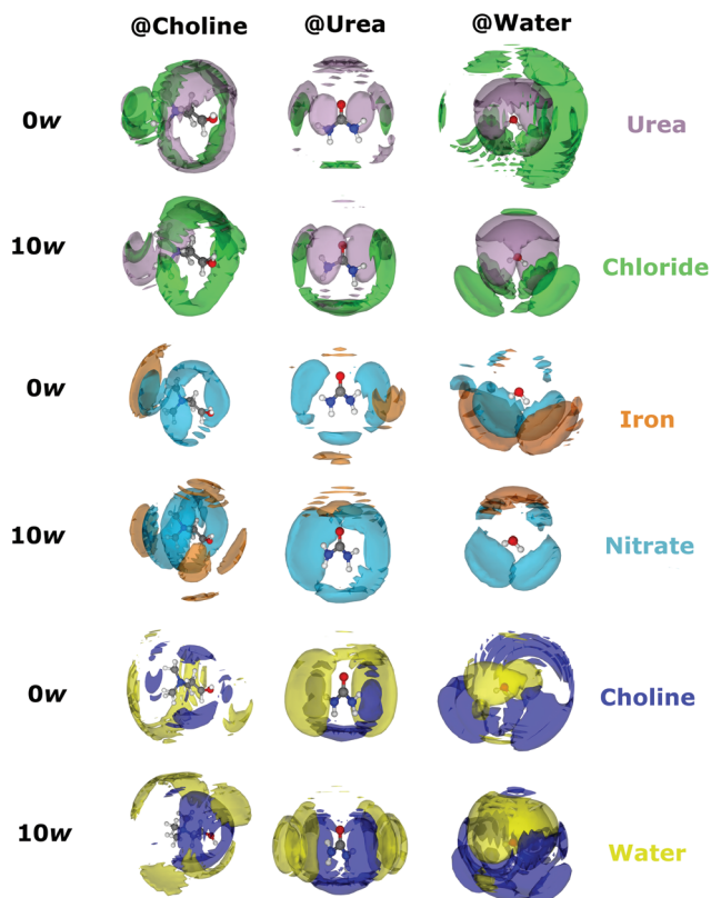
Fig. 3 SDF plots showing most likely 3D configurations of chloride, iron, nitrate, choline, and water molecules, in both the pure and in the hydrated DES in the presence of iron nitrate nonahydrate. Isosurfaces are universally plotted at the 7.5% probability level to facilitate comparison of the degree of order.
