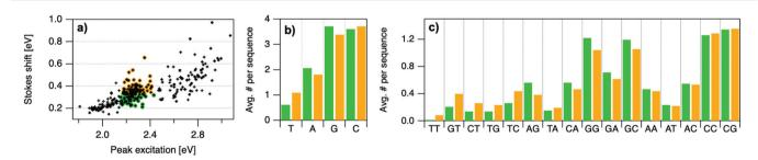
Fig. 6 (a) Indication of low SS (green) and high SS (orange) categories, separated at the median value of SS = 0.336 eV. b, (c) Motifs are sorted left to right in order of greatest relative difference between orange and green bars.
