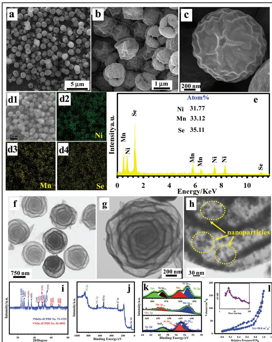
**Fig. 2** (a–c) FE-SEM images of MSNMSeHS. (d1–d4) EDS mapping of MSNMSeHS. (e) EDX spectrum of MSNMSeHS. (f–h) TEM images of MSNMSeHS. (i) XRD pattern of MSNMSeHS. (j) Survey spectrum of MSNMSeHS. (k) Ni 2p, Mn 2p, and Se 3d XPS spectra of MSNMSeHS. (l) BET curve of MSNMSeHS and its corresponding BJH plot (inset).
