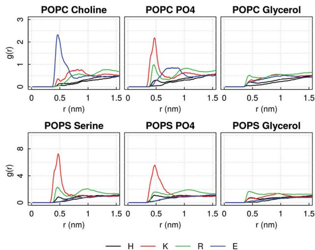
**Fig. 12** SIRAH simulation of AM- $\beta$ -annulus capsule on a bacterial model membrane: Radial distribution function of AM- $\beta$ -annulus charged amino acids around typical moieties of lipids heads, averaged over the time simulated after the capsule binding.
