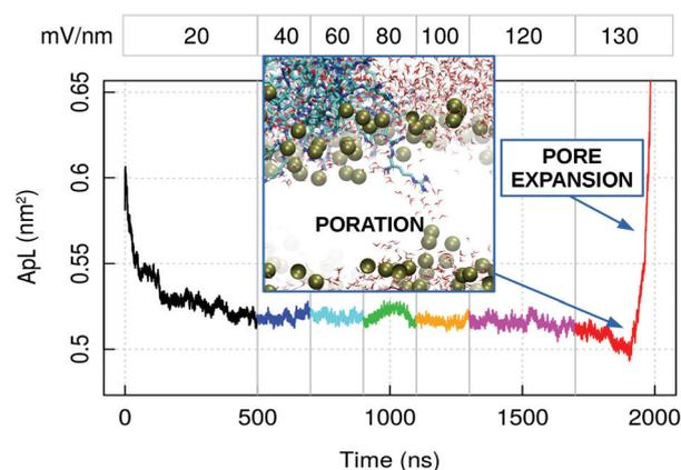
**Fig. 7** Atomistic simulation of capzip pentagonal unit on model bacterial membrane (512 lipids) with increasing applied external electric field: average area per lipid (ApL). The numbers at the top indicate the magnitude of the field in mV nm<sup>-1</sup>. The inset shows the poration event: Lipid boundaries in surface representation, peptides and water molecules in bond representation [VMD software<sup>108</sup>]. The increase in ApL after pore formation is due to the pore expansion.
