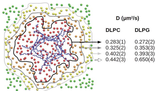
**Fig. 6** Atomistic simulation of capzip pentagonal unit on model bacterial membrane (512 lipids): local lateral diffusion computed along 500 ns for DLPC and DLPG lipids which, at the initial time, are at a distance smaller than 1 nm (red), 2 nm (orange) or 3 nm (yellow) from the peptide or larger than 3 nm (green), centring the trajectory around the Protein COM (blue) [VMD software<sup>108</sup>].
