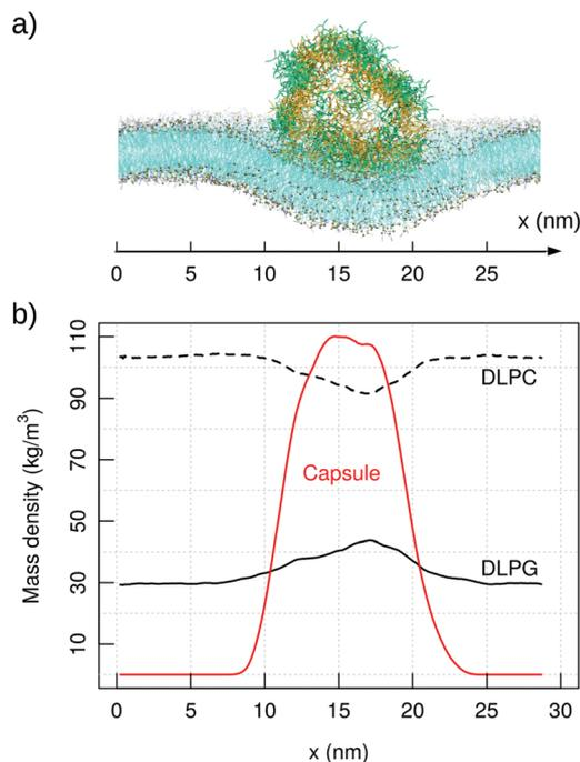
**Fig. 8** MARTINI simulation of capzip capsule on bacterial model membrane (10  $\mu\text{s}$ ): (a) snapshot of the final configuration (capsule in stick representation, outer and inner layer in green and yellow respectively; lipids in line representation and phosphate beads in golden van der Waals – VMD software<sup>108</sup>); (b) corresponding mass density of capzip, DLPC and DLPG along the x-axis, averaged on the last  $\mu\text{s}$  of simulation.
