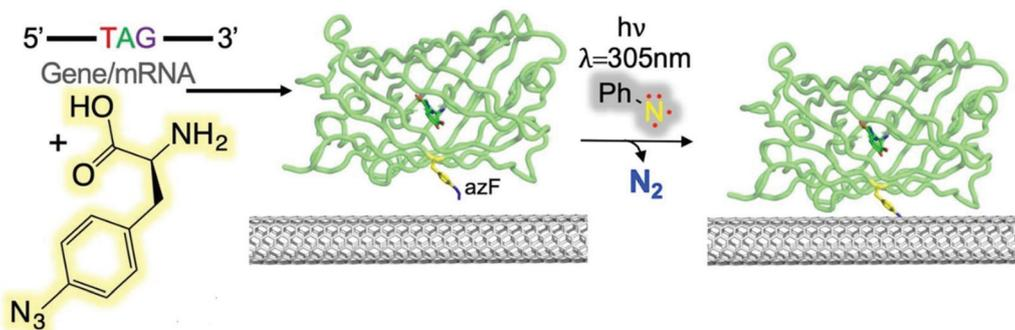
**Fig. 13** Direct protein attachment to CNTs via phenyl azide photochemistry. Scheme of photochemical insertion of a protein via genetically encoded phenyl azide chemistry. Reprinted with permission from Thomas *et al.*, *Bioconjugate Chem.*, 2019, **3**, 584.
