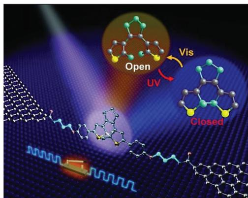
**Fig. 8** Schematic of a graphene-diarylethene-graphene junction that highlights the expansion of the molecular bridge by methylene groups. Reprinted with permission from Jia *et al.*, *Science*, 2016, **352**, 1443. Copyright 2016 AAAS.
