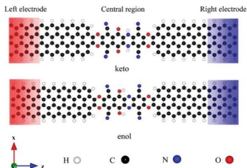
**Fig. 10** Schematic of investigated molecular junctions, where the keto and enol molecules are covalently fused into the zGNR electrodes. The left and right electrodes are denoted by the red and blue rectangles, respectively. Reprinted with permission from Wang *et al.*, *Nano Lett.*, 2018, **31**, 17650. Copyright 2018 American Chemical Society.
