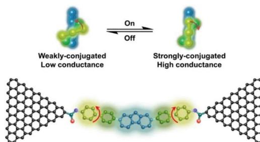
**Fig. 9** Schematic of conformational transition of terphenyl units between strongly conjugated and weakly-conjugated states and corresponding hexaphenyl aromatic chain single-molecule junctions. Reprinted with permission from Xin *et al.*, *Nano Lett.*, 2017, **17**, 856. Copyright 2017 American Chemical Society.
