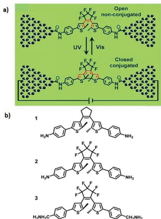
**Fig. 7** (a) Switching of graphene-diarylethene junctions. (b) Molecular structures of three photochromic diarylethene. Reprinted with permission from Jia *et al.*, *Angew. Chem., Int. Ed.*, 2013, 52, 8666. Copyright 2013 Wiley-VCH Verlag GmbH & Co. KGaA.
