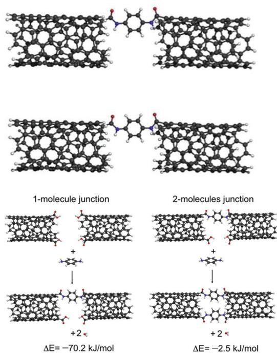
**Fig. 12** Schematic of a PPD (*p*-phenylenediamine)-linked molecular junction and reactions of formation for linear junctions with one and two bringing molecules. Reprinted with permission from Zhu *et al.*, *J. Am. Chem. Soc.*, 2016, **9**, 2905. Copyright 2016 American Chemical Society.
