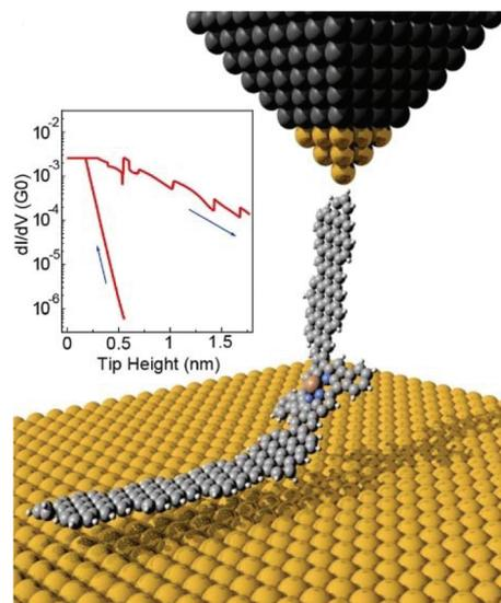
**Fig. 11** Illustration of the target experimental geometry. The inset shows a typical conductance–distance plot simultaneously recorded during tip approach and retraction. Reprinted with permission from Li *et al.*, *Nano Lett.*, 2019, **19**, 3288. Copyright 2019 American Chemical Society.
