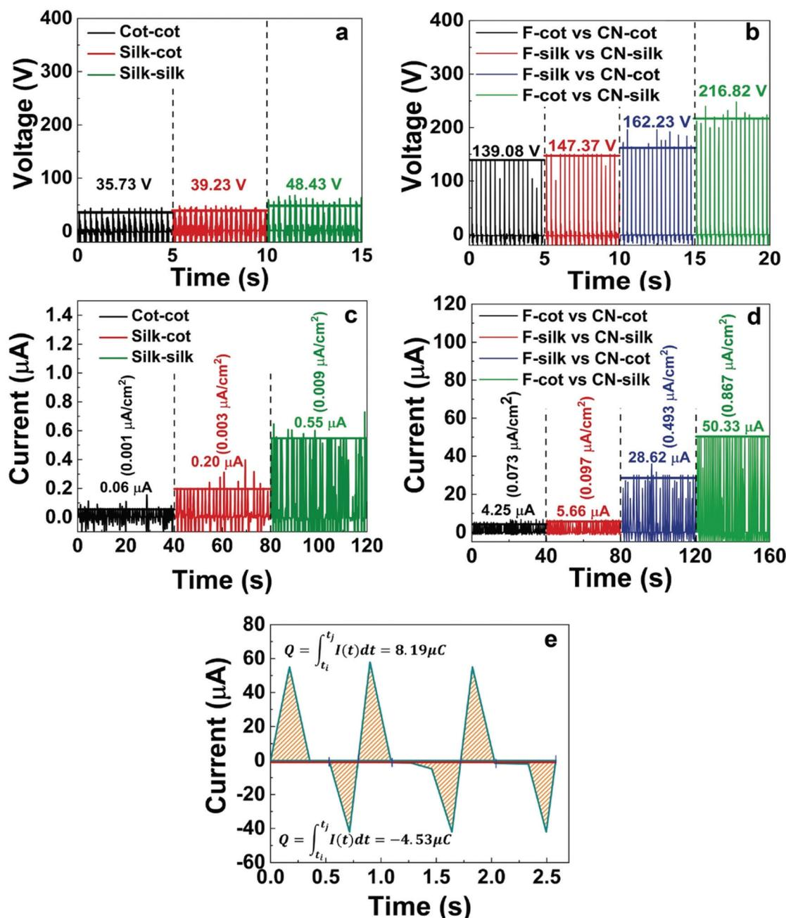
Fig. 6 (a) Output voltage of pristine-TENGs, (b) output voltage of N-TENGs, (c) output current of pristine-TENGs, (d) output current of N-TENGs and (e) three movement cycles of the  $I_{sc}$  signal of F-cot/CN-silk with the average calculated surface charge.
