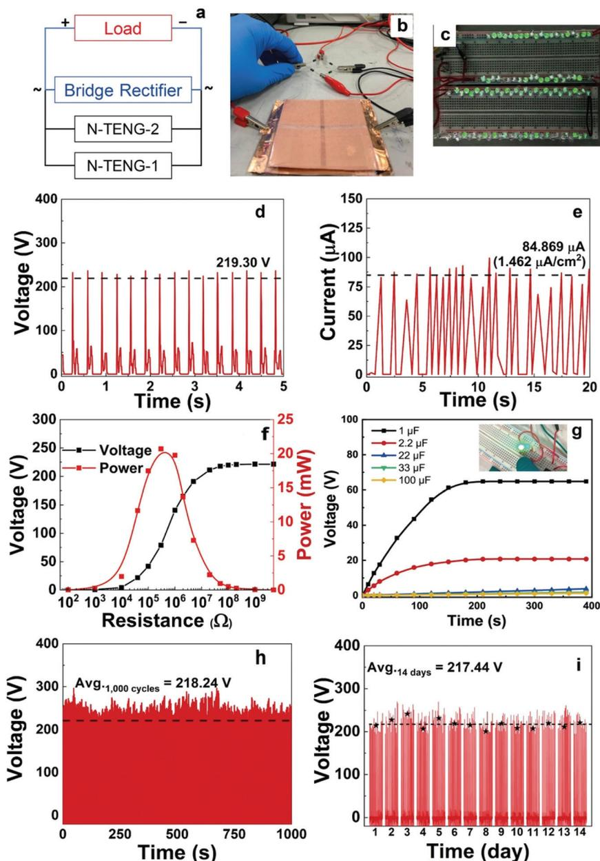
**Fig. 7** (a) Circuit diagram of the double stacked N-TENGs, (b) photograph of double stacked TENG devices connected to a rectifier, (c) photograph of the TENG connected to power 100 LEDs, (d) output voltage, (e) output current, (f) output voltage and output power density when connected to an external load resistance, (g) charging curves of capacitors ranging from 1 to 100  $\mu\text{F}$  as a function of time and a LED powered by a charged capacitor (inset), and (h and i) stability test.
