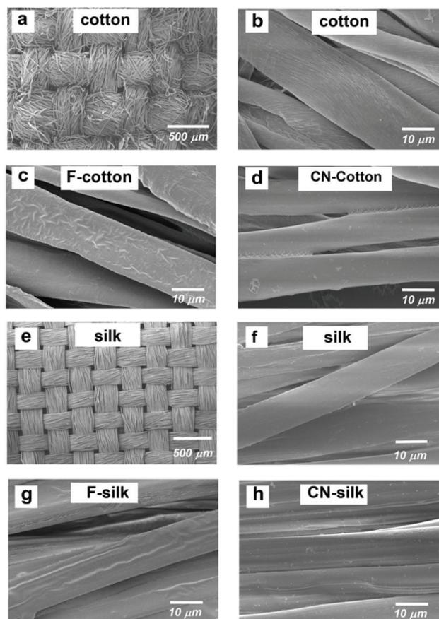
**Fig. 2** (a) and (b) SEM images of plain cotton (500 $\times$ ) and (2000 $\times$ ), (c) fluoroalkylated siloxane coated cotton (F-cotton) (2000 $\times$ ), (d) cyanoalkylated siloxane coated cotton (2000 $\times$ ) (CN-cotton); (e) and (f) SEM images of plain silk (500 $\times$ ) and (2000 $\times$ ), (g) fluoroalkylated siloxane coated silk (F-silk) (2000 $\times$ ) and (h) cyanoalkylated siloxane coated silk (CN-silk) (2000 $\times$ ).
