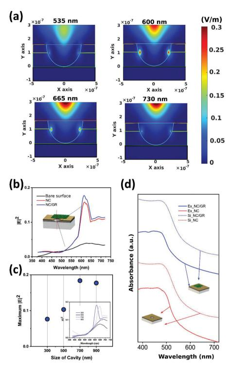
Fig. 4 FDTD simulation of surface intensity absorbance and electrical field of the proposed platform. (a) The 2D contour of the maximum value of the absolute electrical field in the three platforms in the broadband wavelength. (b) Maximum of the absolute electrical field in the three platforms in broadband wavelength. (c) The maximum electrical field for different sizes of the cavity. (d) Experimental and simulation comparison of absorbance of platforms with and without graphene.
